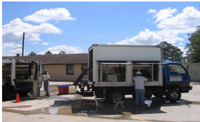
Figure 1. MIP and DPT in action. Direct push rig is on the left and a data acquisition vehicle housing the MIP field computer and GC detectors is on the right.
