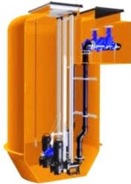
Figure 6: Schematic of a prefabricated submersible lift station. This is a duplex station since it has two pumps. Triplex stations have three pumps.
