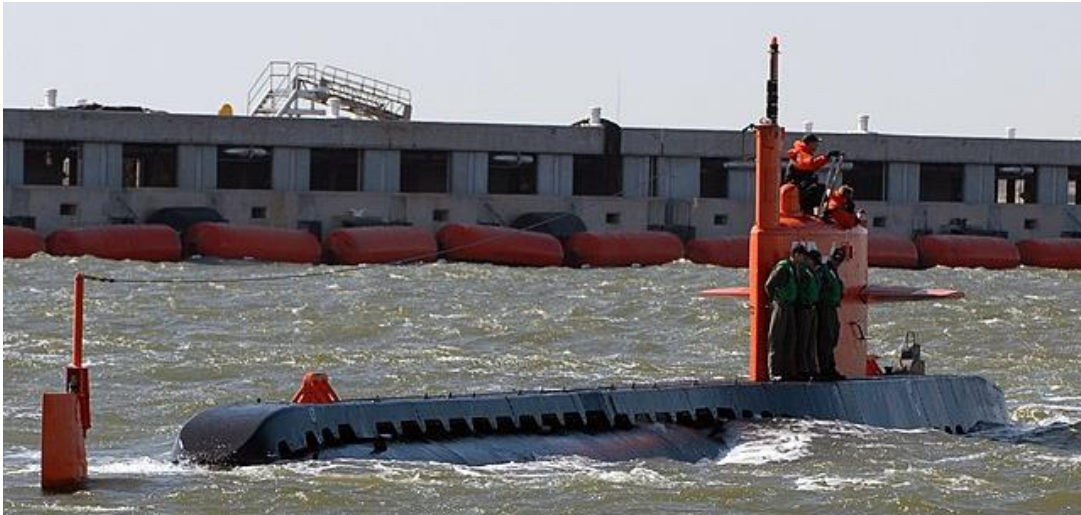
Figure 18: U.S. Navy Nuclear Research Submarine NR-1. This is a unique nuclear-powered deep submergence research vessel that is also used for deep water salvage and reconnaissance of foreign sunken objects. It was the smallest nuclear submarine in the world.
