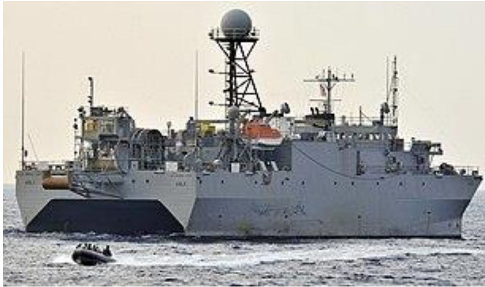
Figure 8: U.S. Navy SWATH T-AGOS ship ballasted down to running draft. Note the large air search radar and the towed array deployment and retrieval equipment on the stern.
