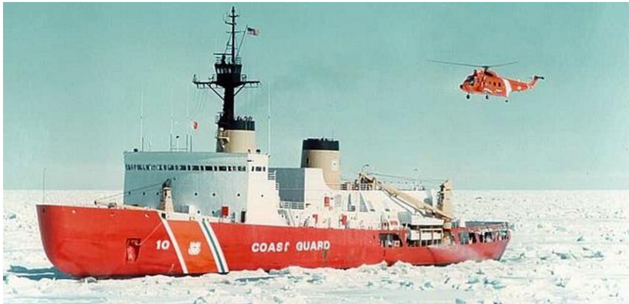
Figure 23: USCG Polar Star Icebreaker, our only operating heavy icebreaker. This one goes to Antarctica and can break ice up to 21 feet thick!
