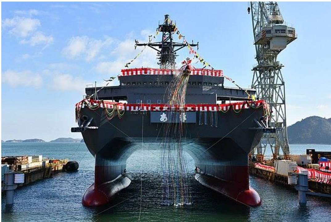
Figure 7: Ocean Surveillance ship AOS 5203 of the Japanese Self-Defense Force (Navy). This is a SWATH hulled vessel
