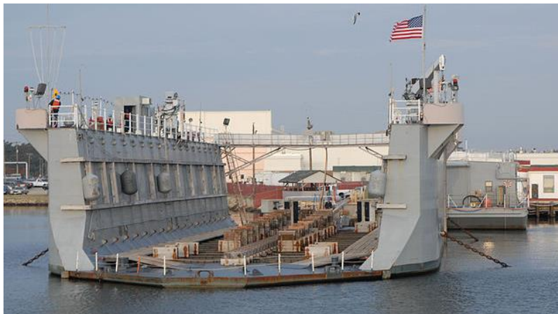
Figure 6: U.S. Navy Floating Drydock AFDL6 preparing to take a ship in on the blocks
