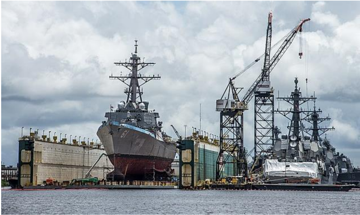
Figure 5: U.S. Navy DDG 61 in the floating drydock at Norfolk, VA. Note the large sonar bulb on the bow and the curved bilge keels on the ship
