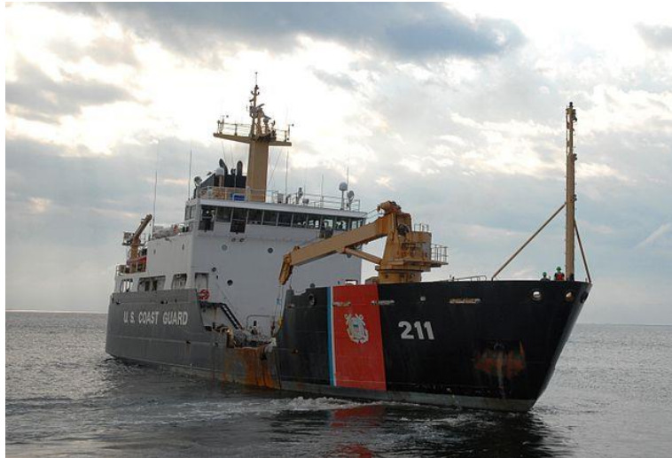
Figure 19: USCG Juniper Class Seagoing Buoy Tender. Coastal Buoy Tenders are similar but smaller.
