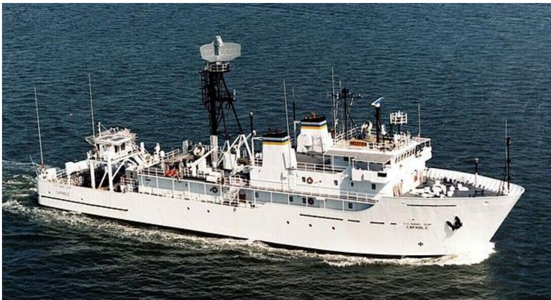
Figure 9: U.S. Navy T-AGOS 16, U.S.S. Capable, an older ocean surveillance ship which has now been converted to do oceanography research. Note the large air search radar for early warning of incoming aircraft, and numerous tall radio antennas.
