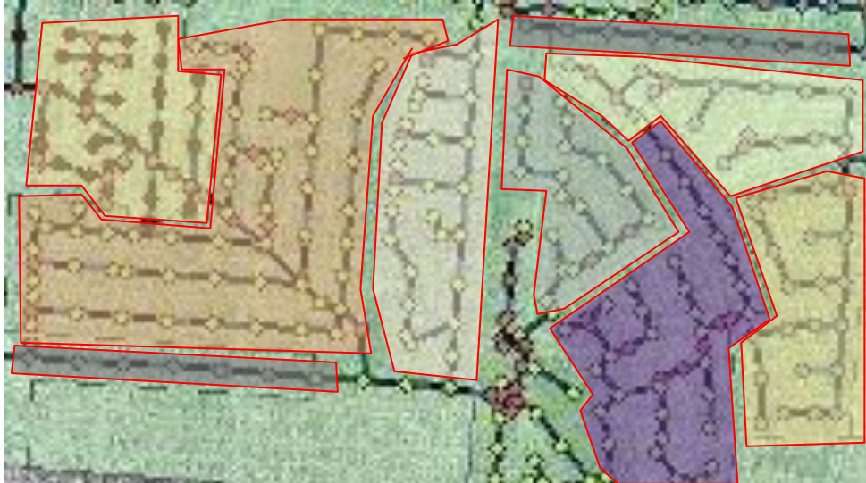
Figure 22: GIS map with sewersheds highlighted in red. When defining a sewershed, it is helpful to make the area as large as possible with the flow still going through a single path such as a manhole or lift station.
