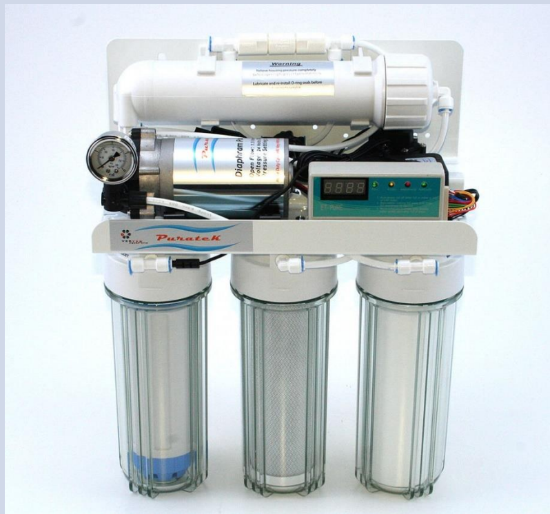
Figure 14: 4-Stage 100 gpd RO Water System with (3) prefilters (carbon and sand) at the bottom, a booster pump (silver) and a RO De-Ionizing Filter (white).
