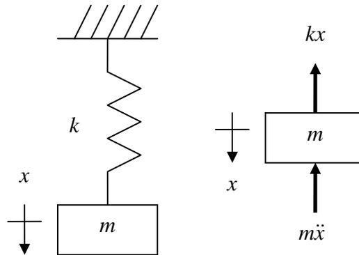
Figure 1.1.3: Single degree of freedom, undamped lumped parameter model (left); free body diagram (right).
