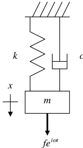
Figure 1.2.1: Single degree of freedom, lumped parameter model (damped with force).
