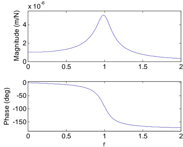
Figure 1.2.2: Magnitude and phase for example single degree of freedom system.
