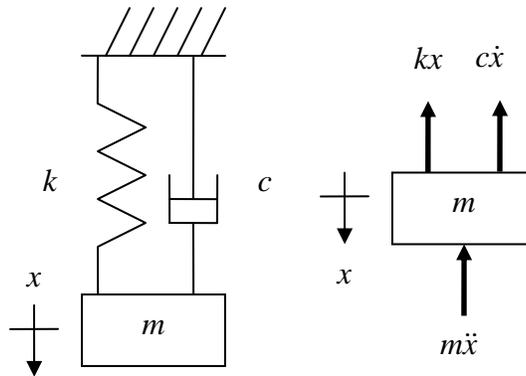
Figure 1.1.5: Single degree of freedom, damped lumped parameter model (left); free body diagram (right).
