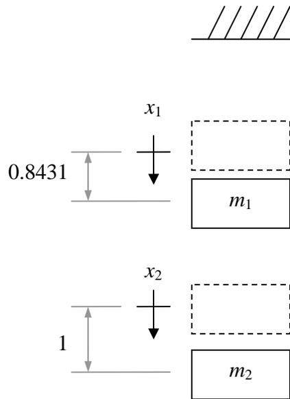
Figure 1.3.2: Mode shape 1 normalized to coordinate 2.
