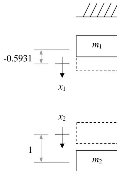
Figure 1.3.3: Mode shape 2 normalized to coordinate 2.
