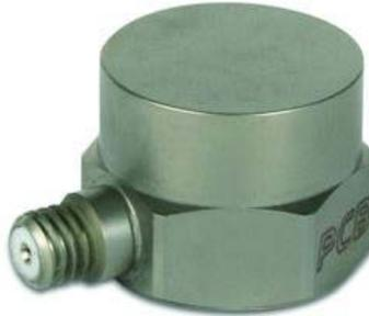
Figure 1.6.3: Example accelerometer with 10 mg mass and 0.5 Hz to 5 kHz measurement bandwidth. Many sizes are available for various applications [9].
