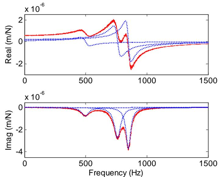
Figure 1.5.4: Example tool point and three modal coordinate FRFs determined by peak picking approach.
