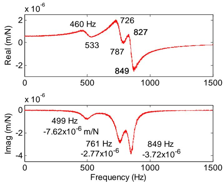
Figure 1.5.3: Three degree of freedom peak picking example with required frequencies and amplitudes identified.
