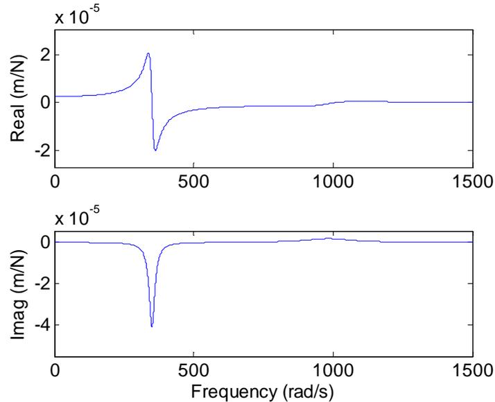
Figure 1.4.3: The real and imaginary parts of the cross FRF are obtained by scaling the two modes by the corresponding mode shape and summing the results.
