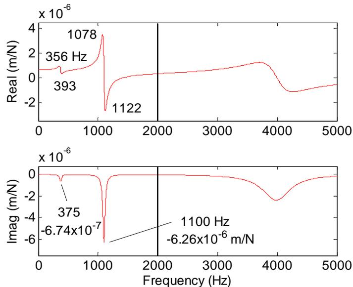
Figure 1.5.7: “Measured” direct FRF for Ex. 1.5.2. The peak picking values are listed within the 2 kHz measurement bandwidth. A 5 kHz frequency range is provided to show the truncated 4000 Hz mode.
