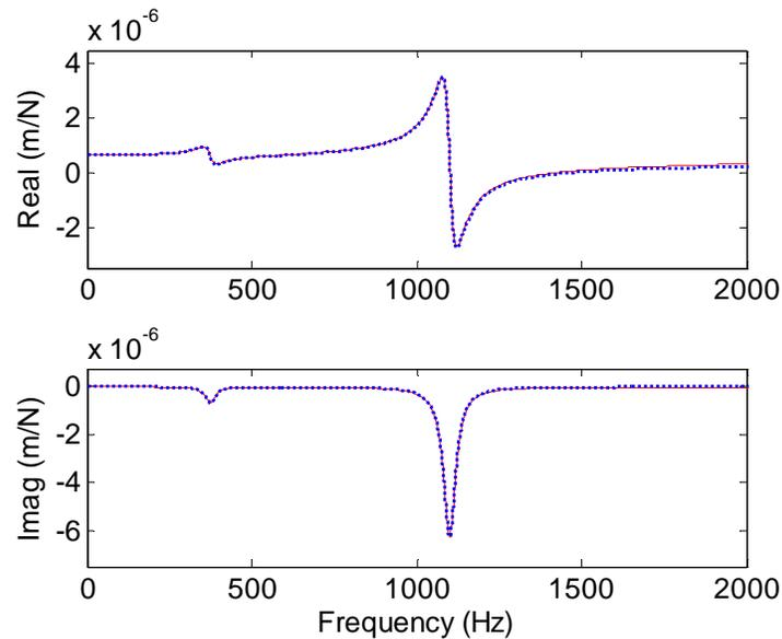
Figure 1.5.9: Result of modal fitting with the addition of a DC compliance term to correct for the truncated mode.
