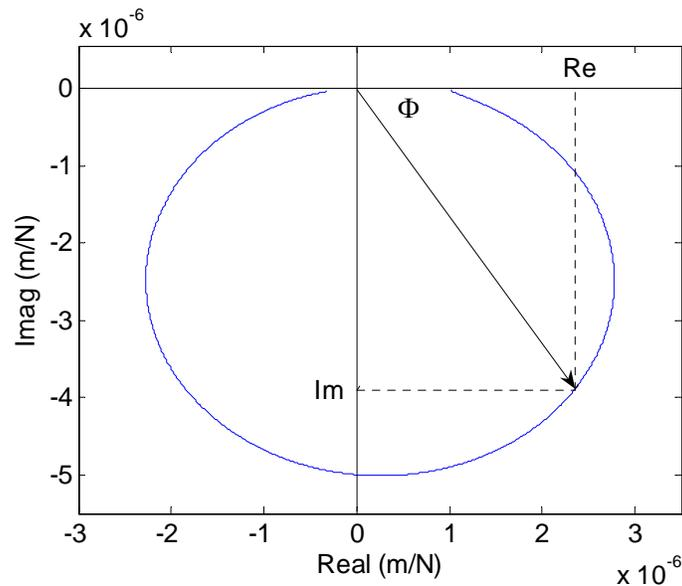
Figure 1.2.5: Vector representation of FRF in the complex plane.
