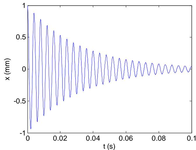
Figure 1.1.1: Damped free vibration example.
