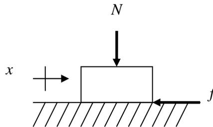
Figure 1.1.4: Coulomb damping occurs due to dry sliding friction between the two surfaces. The normal and friction forces are shown.
