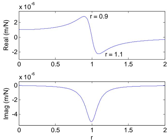
Figure 1.2.3: Real and imaginary parts for example single degree of freedom system.
