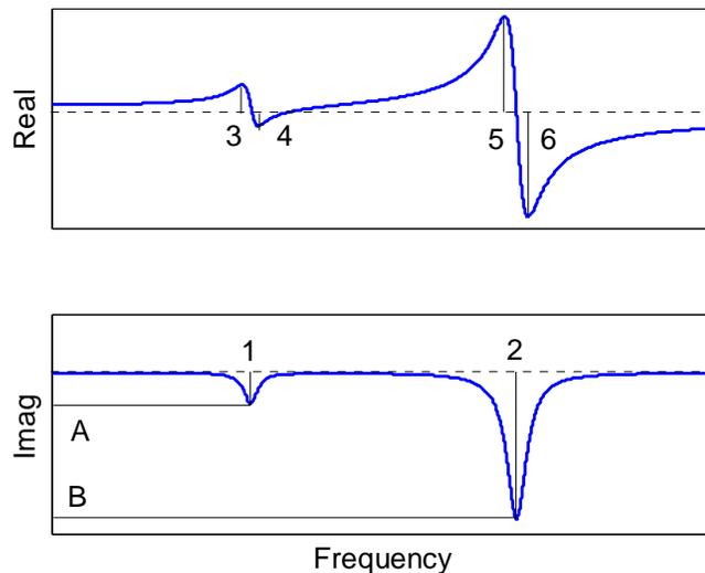
Figure 1.5.1: Two degree of freedom direct FRF with the frequencies and amplitudes required for peak picking identified.
