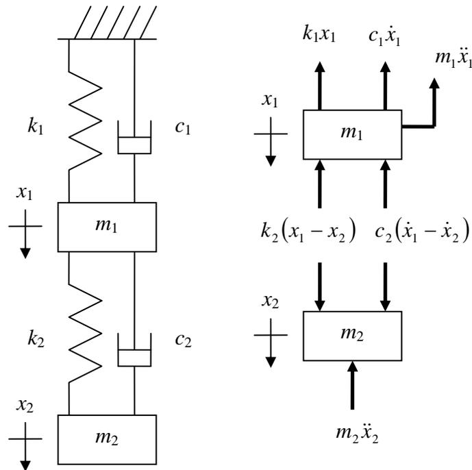
Figure 1.3.1: Two degree of freedom, damped lumped parameter model (left); free body diagram (right).
