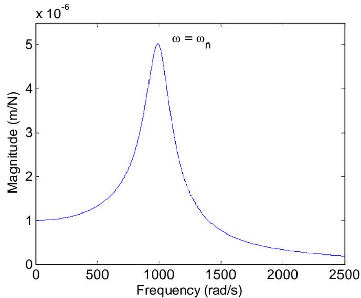
Figure 1.1.2: Example of forced vibration magnitude.
