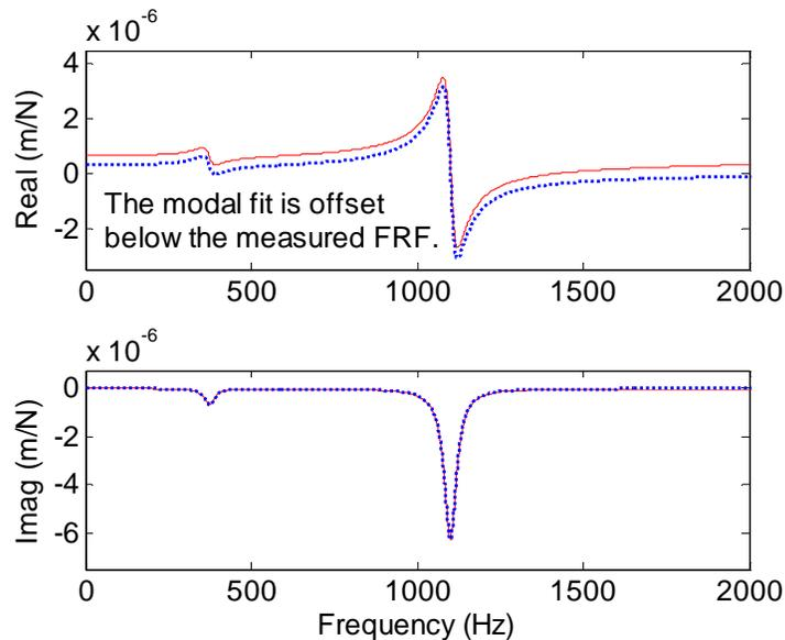
Figure 1.5.8: Result of modal fitting. An offset in the Real part of the fit (dotted line) is observed because the DC compliance of the 4000 Hz mode is not included.
