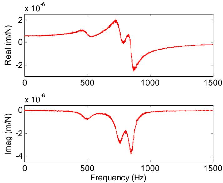
Figure 1.5.2: Example tool point FRF for peak picking exercise.
