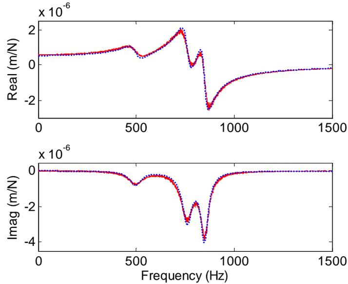
Figure 1.5.5: Example tool point FRF with three degree of freedom modal fit obtained by peak picking.
