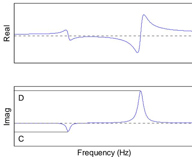
Figure 1.5.6: Two degree of freedom cross FRF with the amplitudes required for model development identified.
