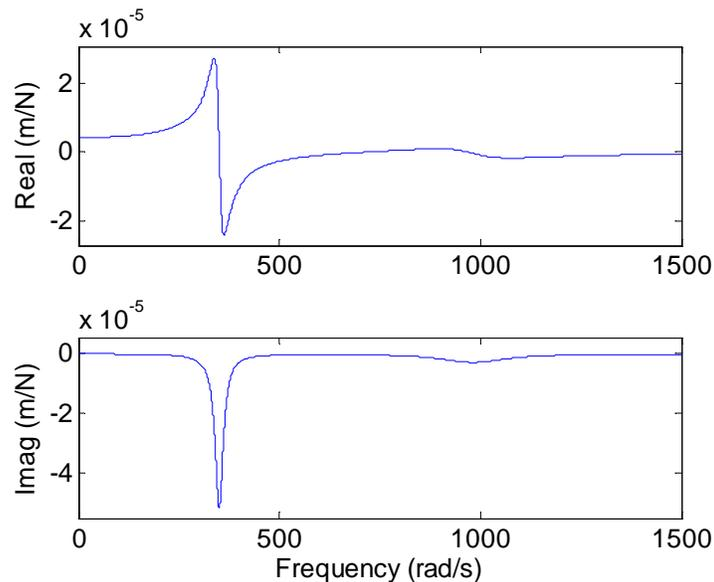
Figure 1.4.2: The real and imaginary parts of the direct FRF are determined from the sum of the modal contributions.
