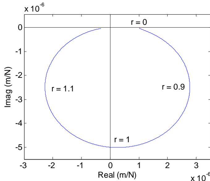
Figure 1.2.4: Argand diagram for example single degree of freedom system.
