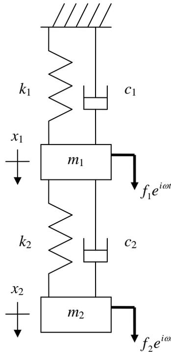
Figure 1.4.1: Two degree of freedom, lumped parameter system (damped with force).
