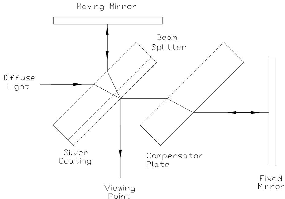
Figure 2.3.2: Michelson interferometer.
