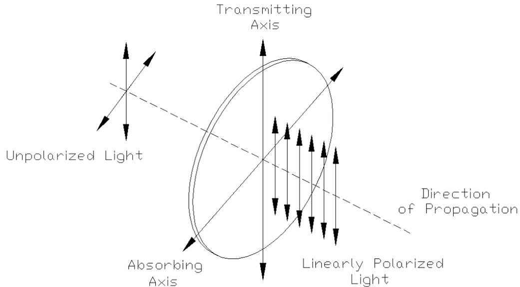
Figure 2.2.1: Polarizing filter.
