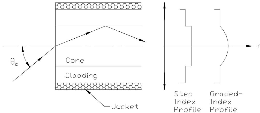
Figure 2.5.3: Refractive index profiles.
