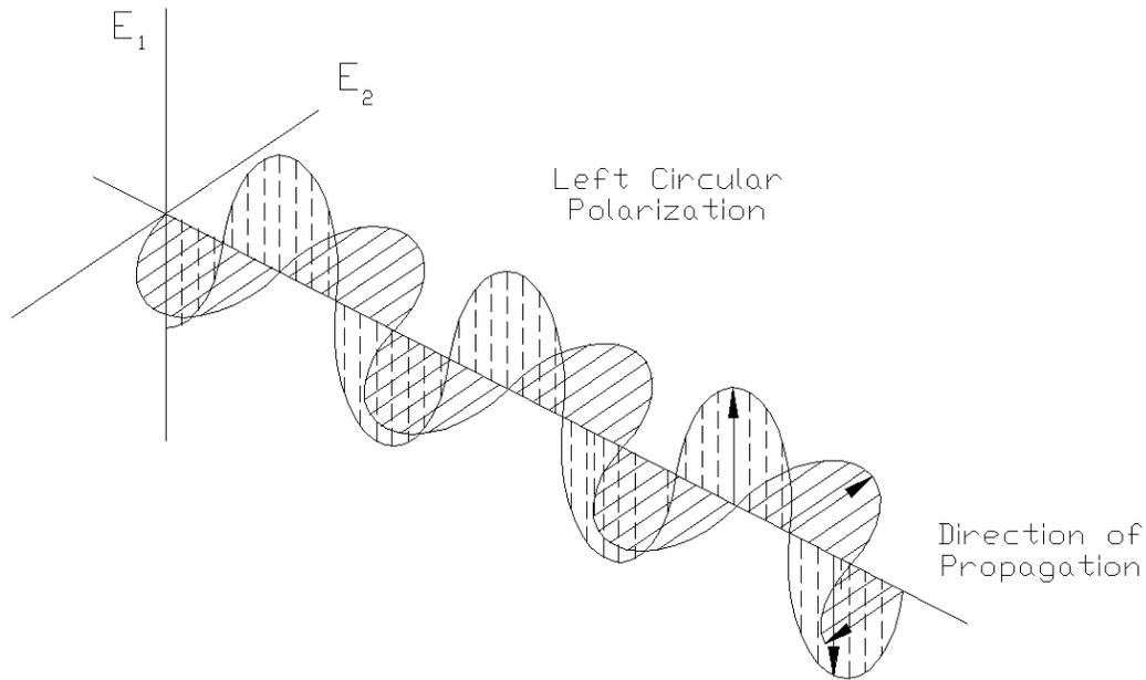
Figure 2.2.3: Left circularly polarized light.
