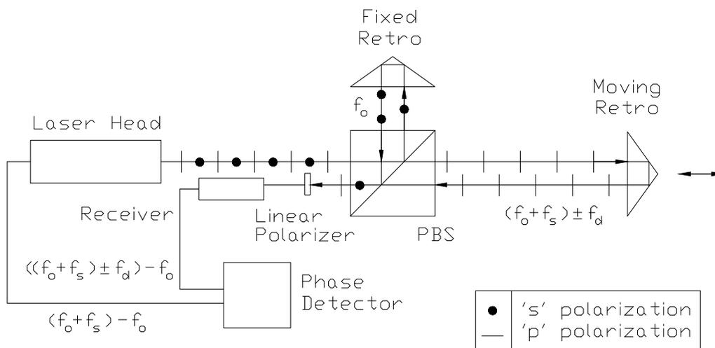
Figure 2.4.6: Linear displacement interferometer.
