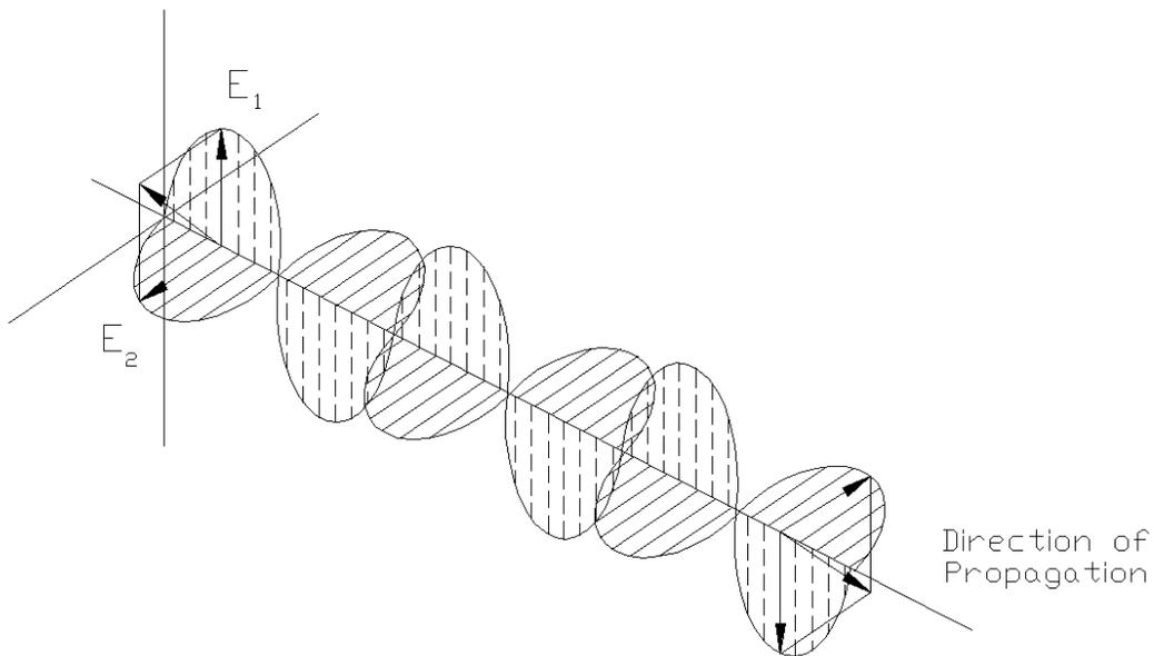
Figure 2.2.2: Linearly polarized light.
