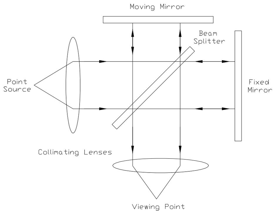
Figure 2.3.3: Twyman-Green interferometer.
