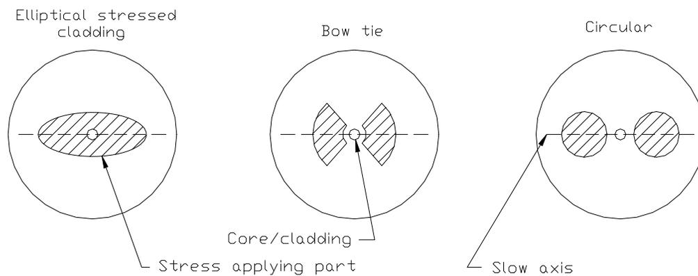
Figure 2.5.4: Single mode fibers.
