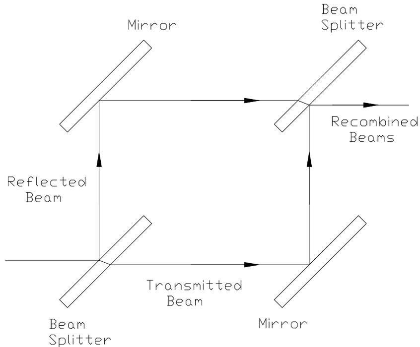
Figure 2.3.4: Mach-Zehnder interferometer.
