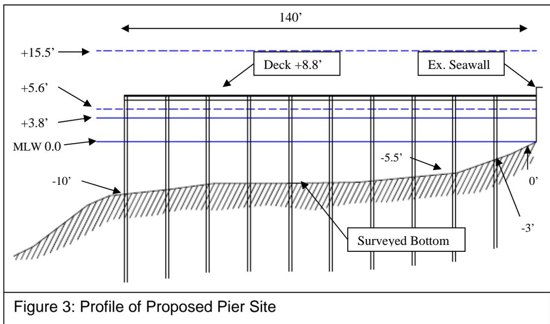
Figure 3: Profile of Proposed Pier Site
