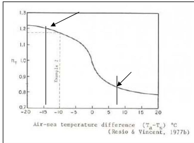
Figure 4: Chart reproduced from COE Shore Protection Manual (Formula 3-14) to find  $R_T$  based on Air / Water Temperature Differential (Note that Temperatures are in Celsius)
