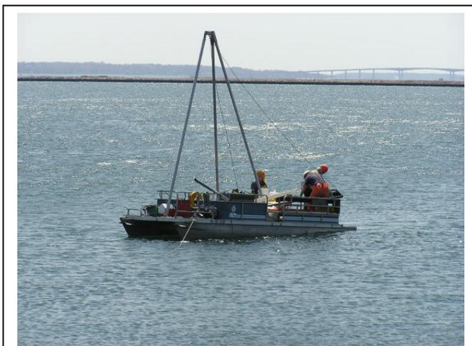
Figure 7: Example of simple floating split-spoon tripod sampling rig
