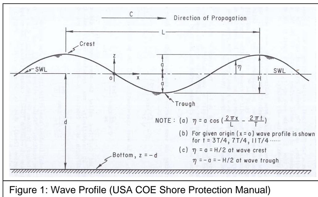
Figure 1: Wave Profile (USA COE Shore Protection Manual)
