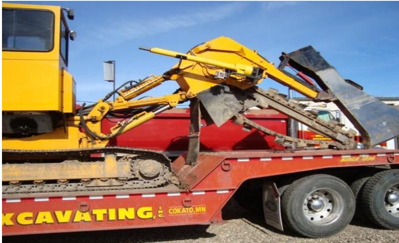
**Figure 15 Heavy duty Minnesota agricultural chain trencher.**
