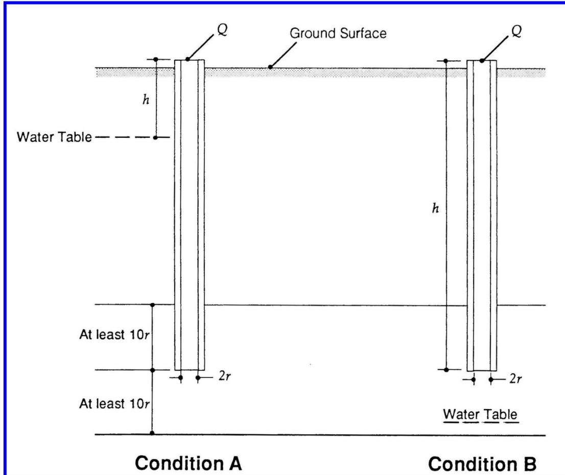
Hydraulic conductivity is calculated from the following equation for both conditions:
