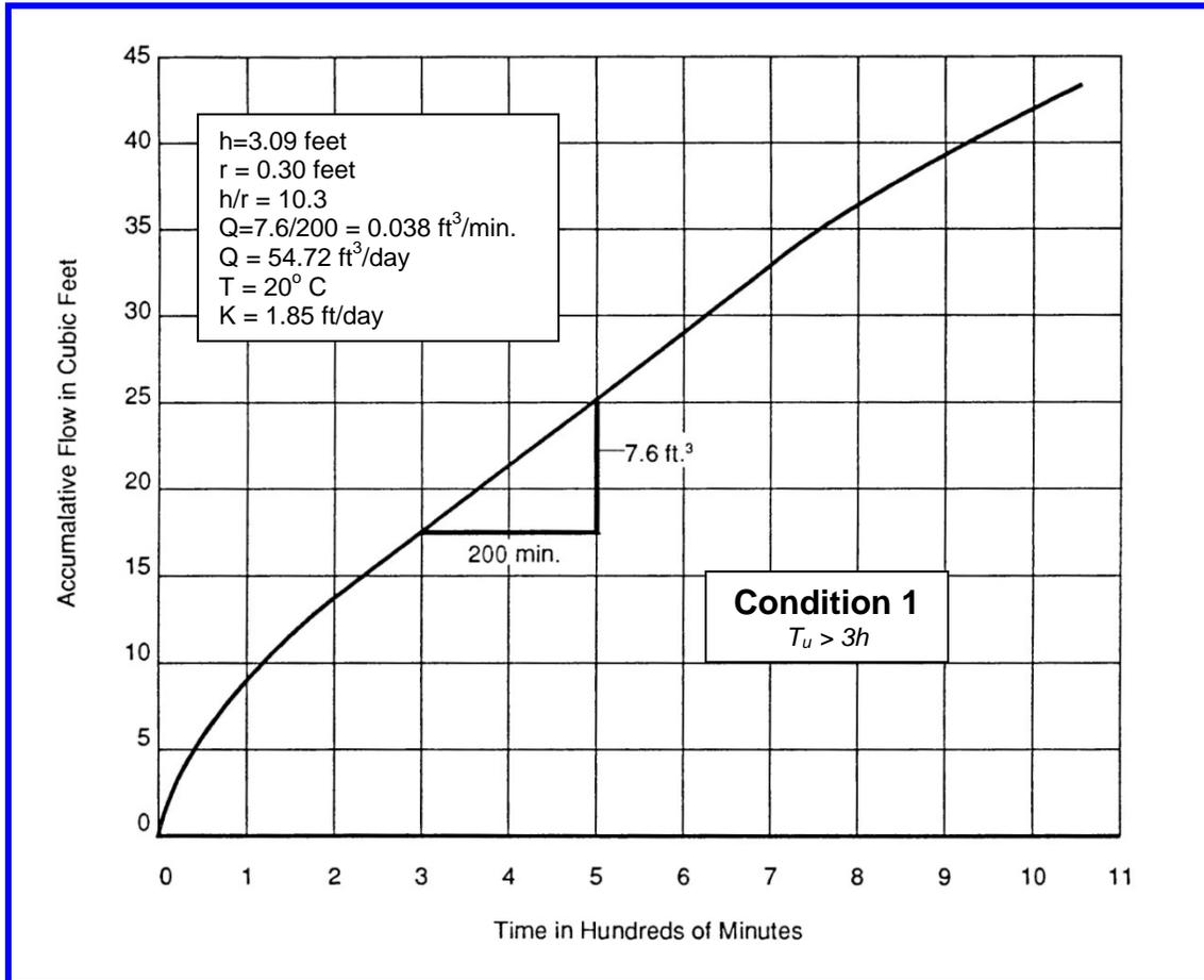
The U.S. Department of the Navy, Naval Facilities Engineering Command (1974) has standard methods of performing variable head tests to estimate the in-situ hydraulic conductivity by means of cased and uncased holes. **Figure 5** summarizes the methods of calculating hydraulic conductivity using the U.S. Department of the Navy methods.
