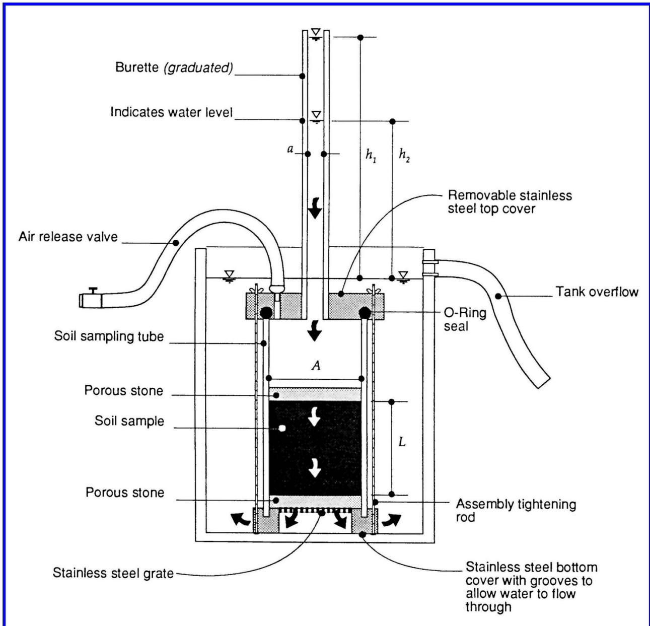
The second method of laboratory hydraulic conductivity measurement involves re-molding a disturbed soil sample, compacting the sample to an estimated in-
