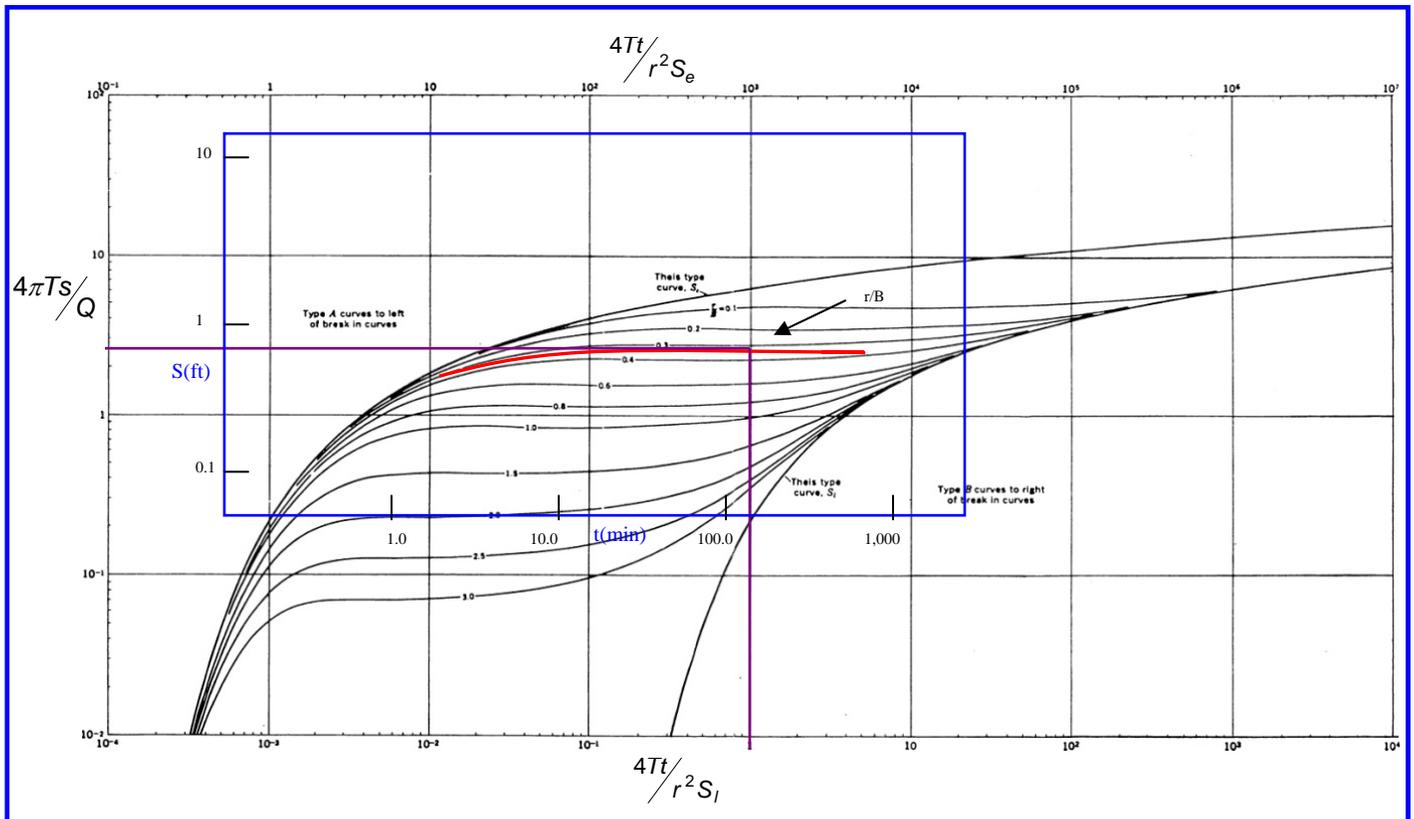
For a pumping test in an unconfined aquifer the red curve above represents the best match of drawdown versus time data for a pump test observation well. The following aquifer conditions and pump test data produced the matching curve:
