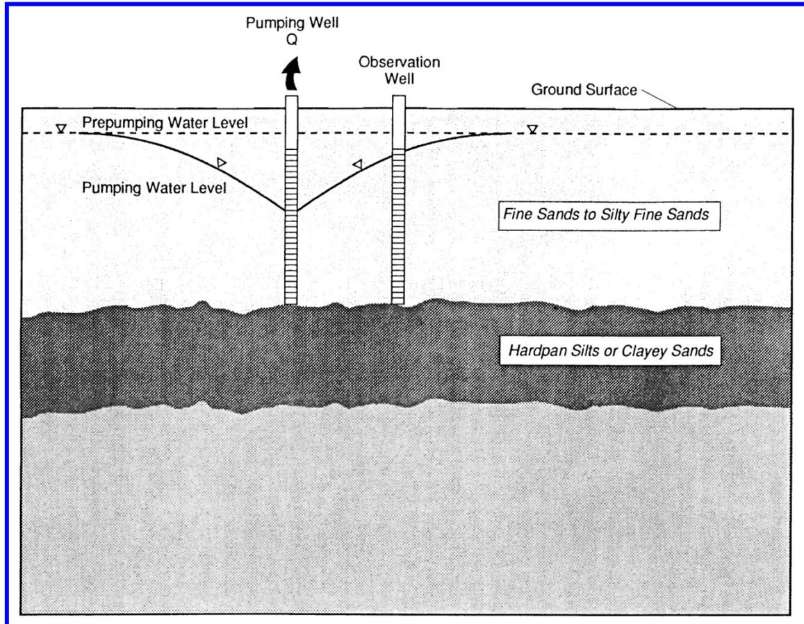
The pumping well and observation well should be installed with the same characteristics (same depth and screen interval). Prior to initiating pumping, the static water level below the top of the casing should be measured in all wells. Then one well should be pumped at as high a rate as possible (to stress the aquifer) and the drawdown below the static water level should be measured in the observation well(s).
