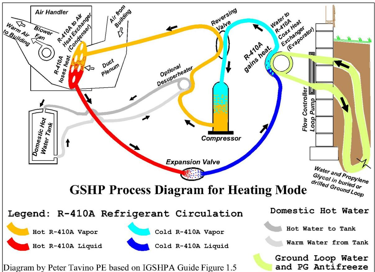
Figure 5 Heat Mode diagram. Similar to Figure 1.5 in the Closed-Loop GSHP Systems Original 1988 Installation Guide distributed by IGSHA.
