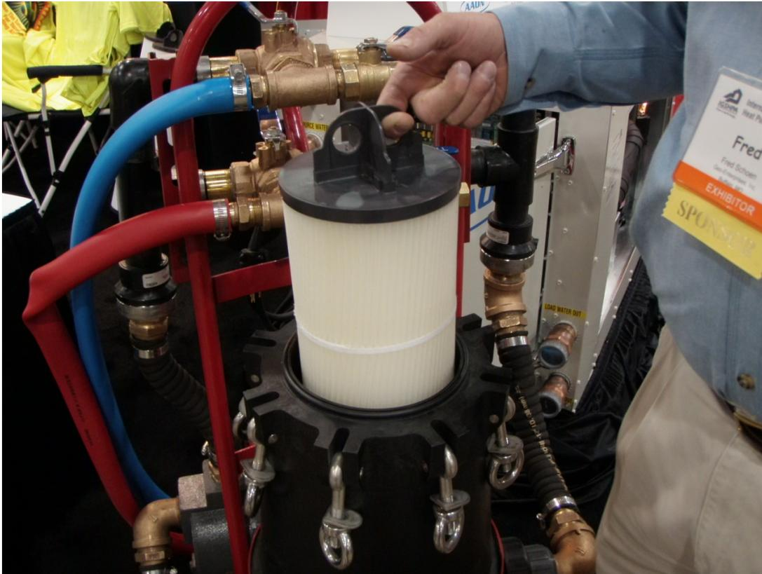
*Figure 18 Removing filter from the flush cart.*
