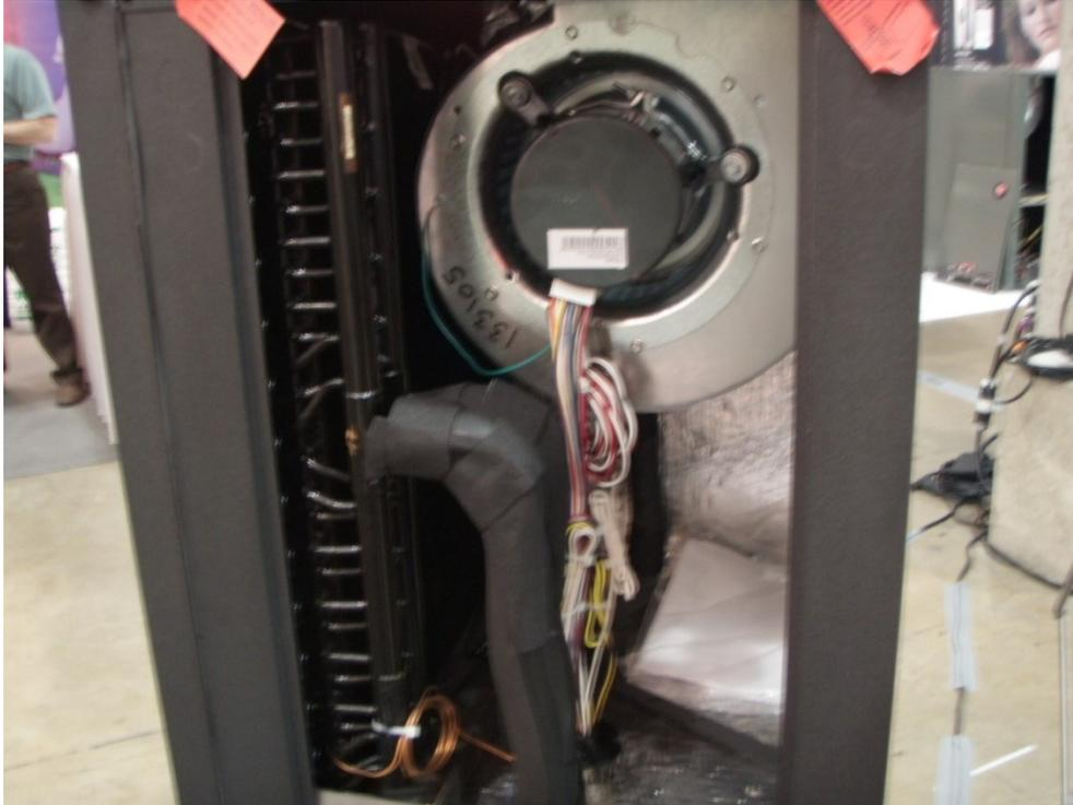
**Figure 9 Humidification / dehumidification assembly located next to the condenser.**
