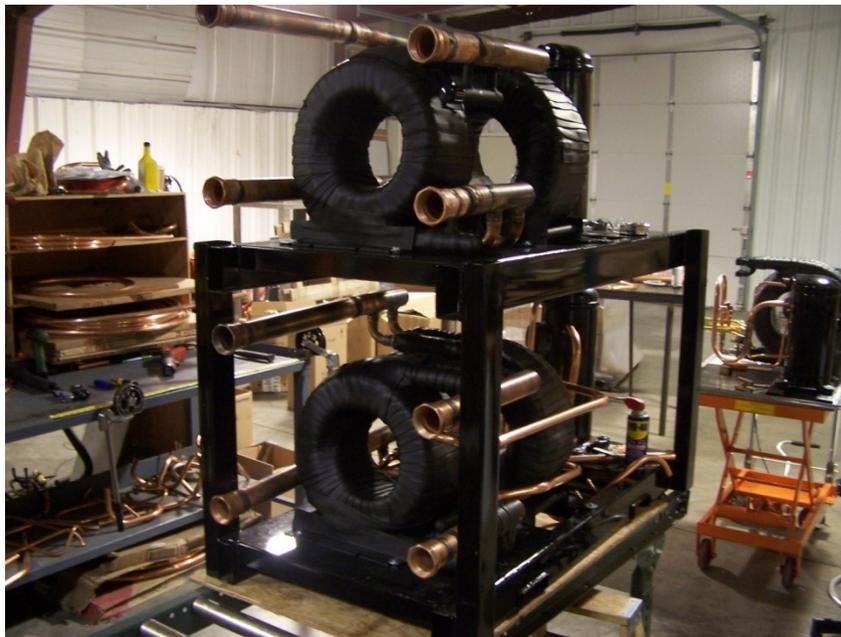
*Figure 26 15-ton water-to-water heat pump. Special thanks to Aaron Sorenson EIT, (now with Bosch) for these photos in fig. 26 and 27, and three earlier ones.*
