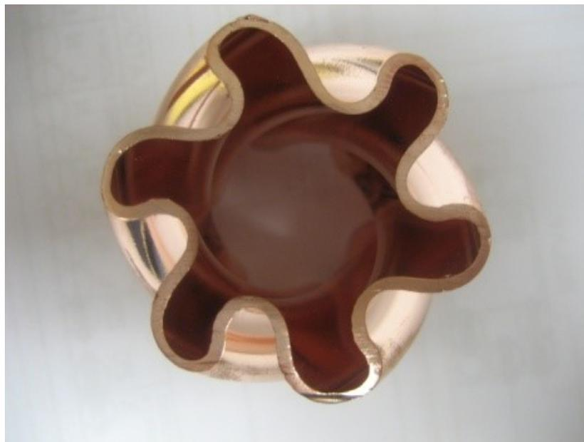
*Figure 13 The way the loop water makes good contact with the R-410A refrigerant within this copper and steel coil is key to efficient GSHP operation.*
