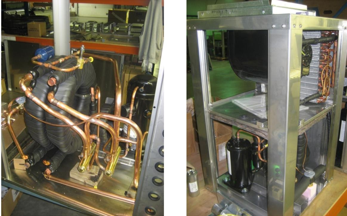
***Figure 27 Heat Pump under construction***
