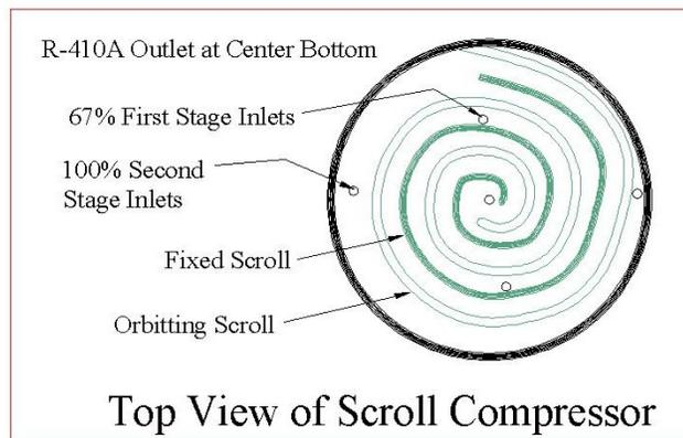
*Figure 29 How scroll compressors operate. <http://www.youtube.com/watch?v=IOL45plqJv4>*
