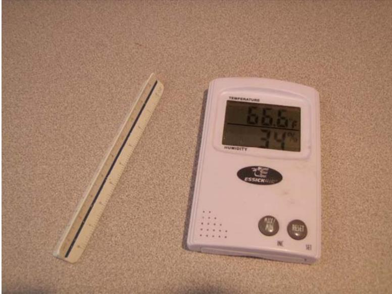
*Dual Display Thermometer / Hygrometer*
