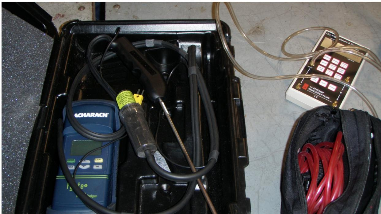
*Portable Carbon Monoxide Detector and a separate DG-700 Digital Manometer*
