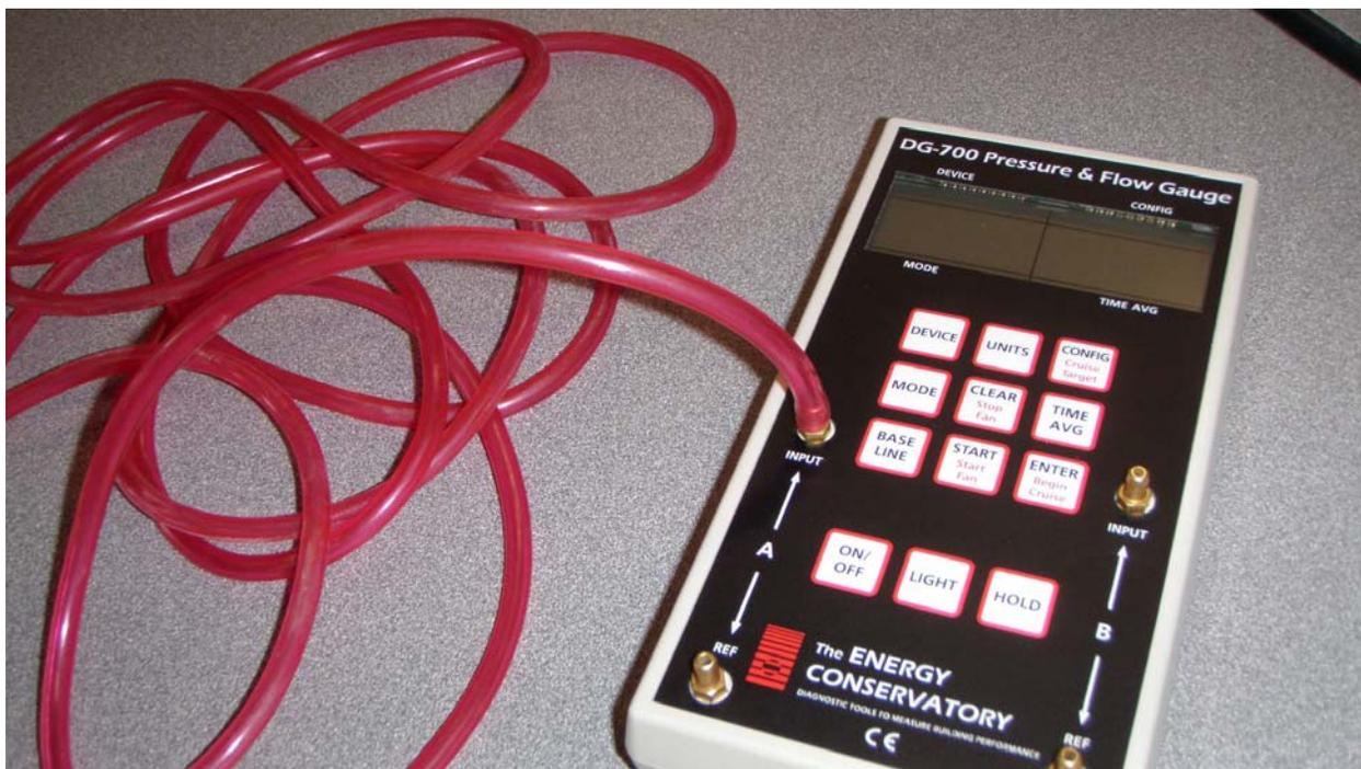
*DG-700 red tubing attached to Channel A for measuring pressure at the end of the tubing .*
