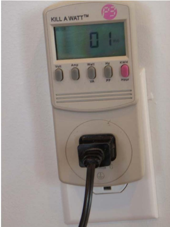
*One watt is being used by the “plug in alarm clock” that is being tested by the Kill A Watt.*
