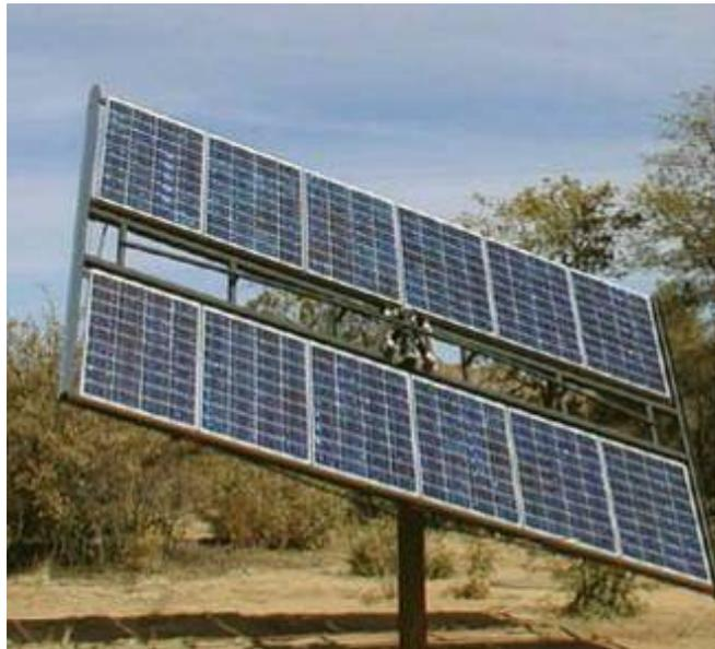
Many of the trackers are advertised as providing a 20 to 30 percent gain in output that the solar panels provide as compared to non-tracking mounts.
