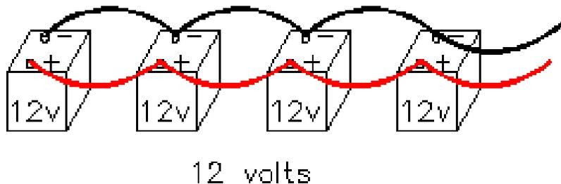
**Remember: Parallel wiring → Voltage stays the same and the Current is additive.**
