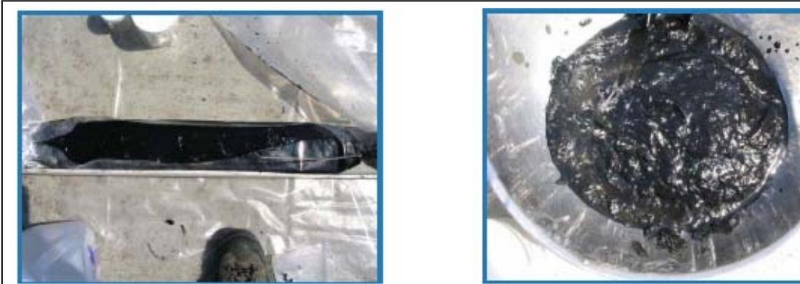
Figure 6: Vibracore Tube liner (Left) opened for sample removal. (Right) sample of typical “soft mud” CSO Outfall sediment.
