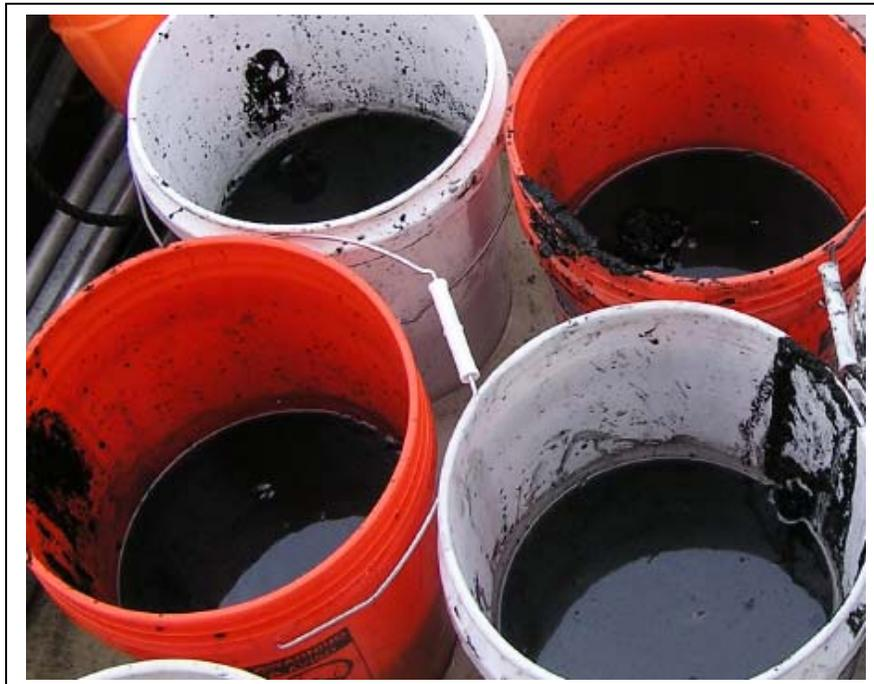
Figure 7: Samples of “fluid” or “soupy” upper sediment layers, Being collected for dewatering “bench tests”
