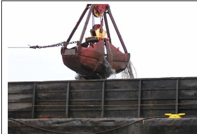
Figure 10: Conventional Clamshell bucket, with rounded digging “nose”, generally used for harder bottom materials
