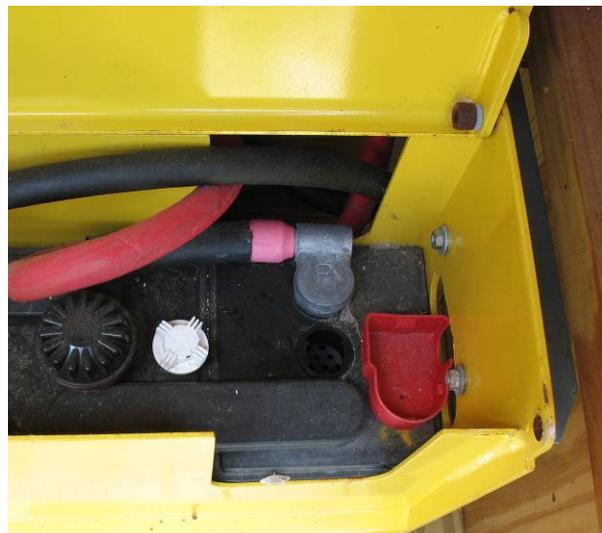
If the batteries do not have vent caps, they are either sealed gel or AGM (Absorbed Glass Mat) batteries. **Sealed Gel** and **AGM** batteries are often used because they have no vents that can release gas during the charging process which allows them to be stored indoors. They are also maintenance free since they don't require someone adding water to them on a regular basis.
