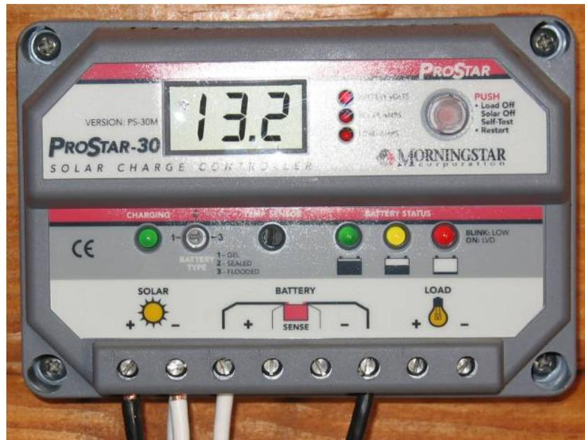
**Max Voltage:** Displays the highest battery voltage recorded since the meter was reset. Using this reading, you can determine the maximum voltage the system experienced since the meter was reset. It will also let you know if an overvoltage condition occurred or if the system is charging at the proper rate.
