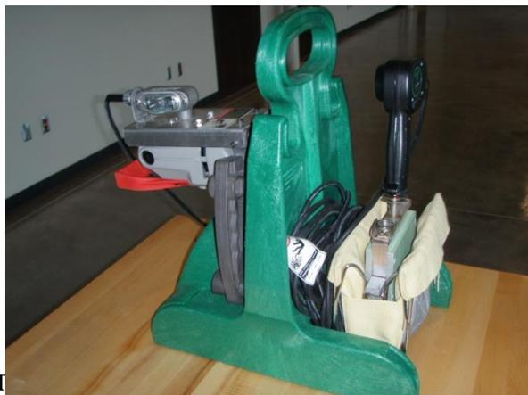
**Figure 31** Left: Butt Fusion, Right: Socket Fusion
