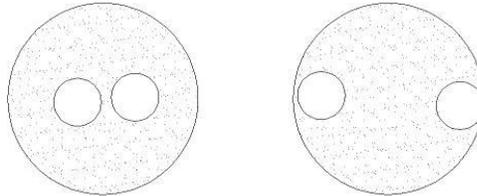
**Figure 17 Cross-sectional Drawing of 1 1/4" loop pipes in a 6" borehole.**
