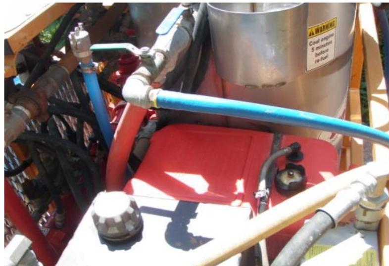
**Figure 23 Water enters the mixing hopper as controlled by the valve.**
