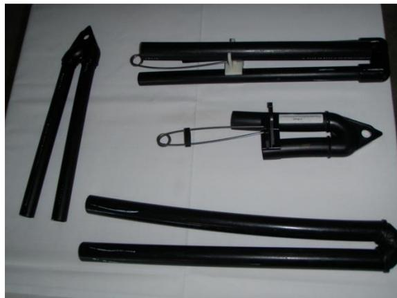
**Figure 10 Left: A Unicoil or U-tube ready to be set into a borehole. Right: Various types of U-bends placed at bottom.**
