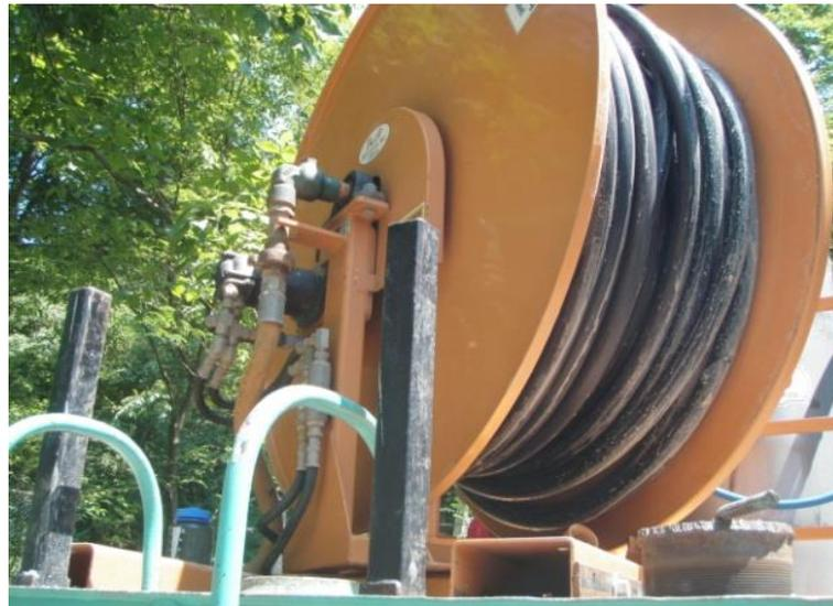
**Figure 26 An electric motor winds the spool to raise the end of the tremie pipe as the grout is added.**
