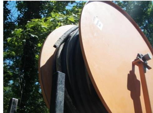
**Figure 19** 1 1/2" HDPE tremie pipe on a spool at the back of the truck. It is connected to the mixer near the supply of bagged silica sand and bentonite grout mix.
