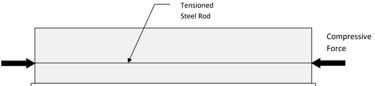
Post-Tensioned Beam After Force Transfer
