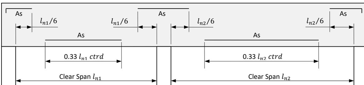
**Minimum Lengths of Bonded Reinforcing**
