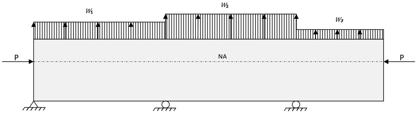
**Equivalent Tendon Loads Applied to Continuous Beam**
