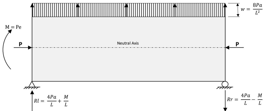
Equivalent Tendon Loads Applied to Beam
