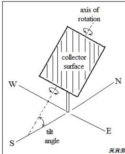
Figure 3. Single axis Tracking Flat-Plate Collector with North-South Axis
