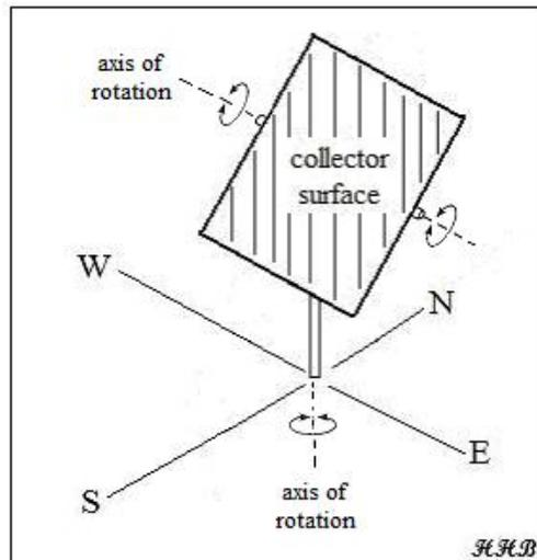
Figure 4. Two-Axis Tracking Flat-Plate Collector
