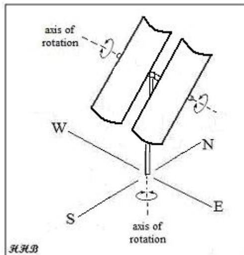
Figure 6. Two-Axis Tracking Concentrator
