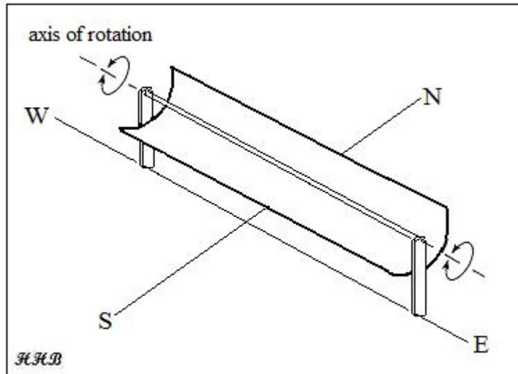
Figure 5. One-Axis Tracking Parabolic Trough with East-West Axis
