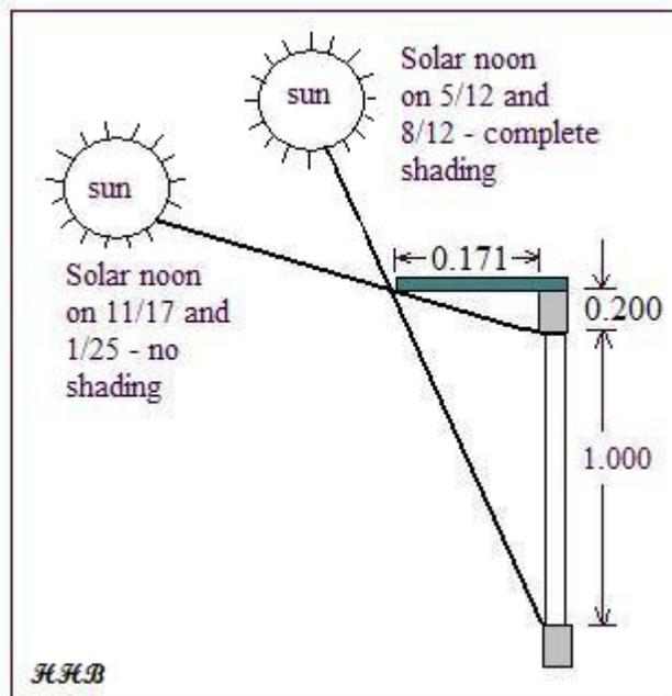
Figure 8. Shading Geometry and Sun Positions for 64° North Latitude
