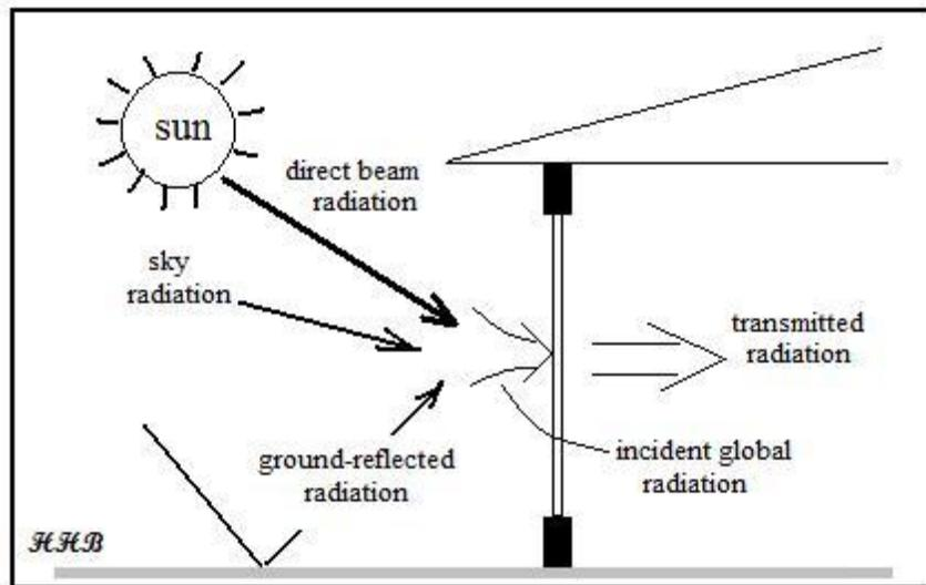
Figure 7. The Components of Global Solar Radiation
