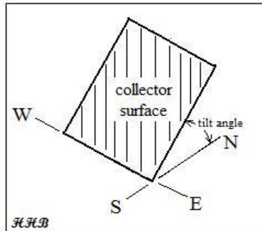
Figure 2. Fixed Tilt Flat-Plate Collector Facing South
