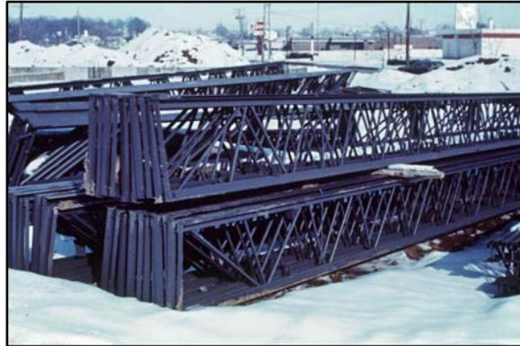
Photo No. 6 - Bar joists ready for delivery
