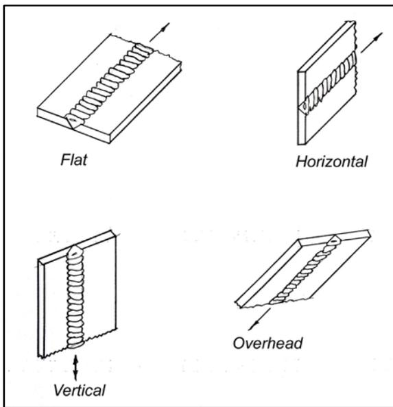
Figure 7 - Weld Positions
