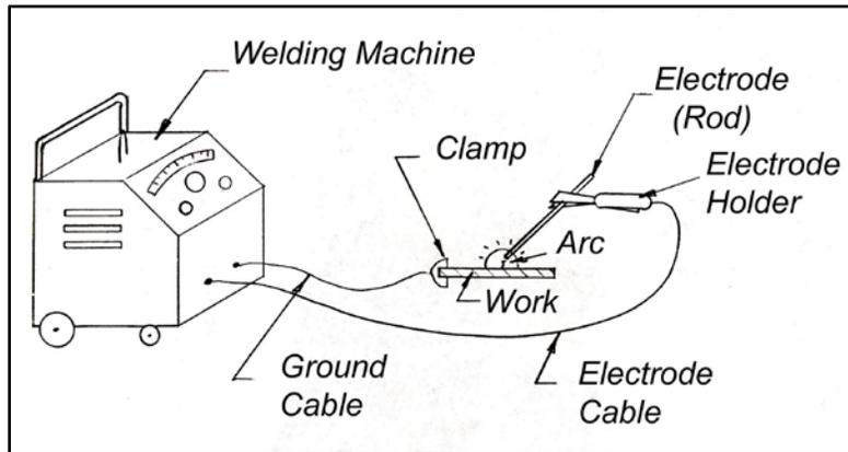
Figure 1 - Depiction of an electric arc welding system
