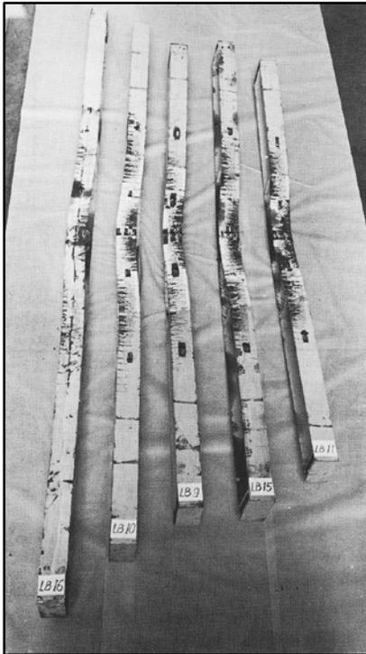
Photo No. 16 - Laterally buckled beams
