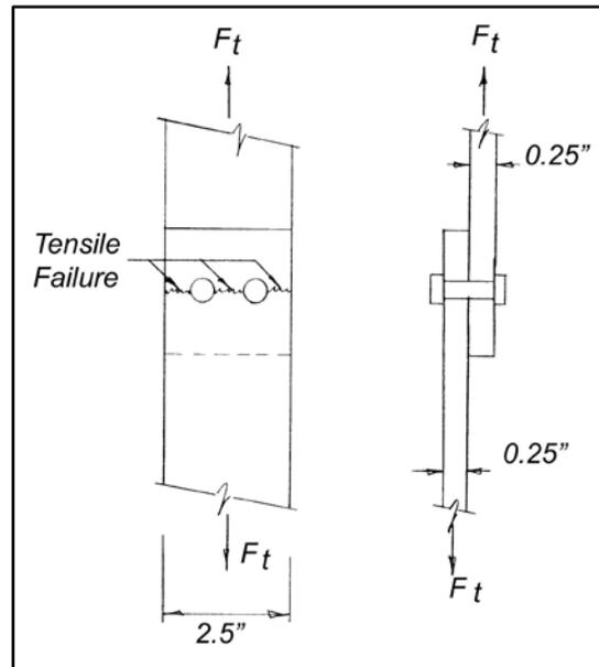
Figure 13 – Tensile failure
