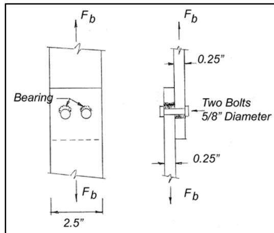
Figure 12 - Bearing failure
