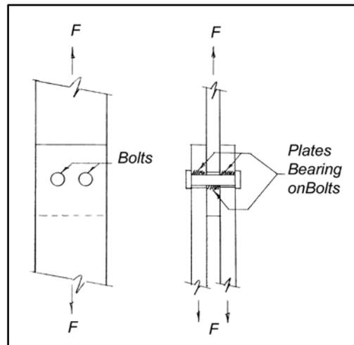
Figure 10 - Bolted Connection - Double Shear
