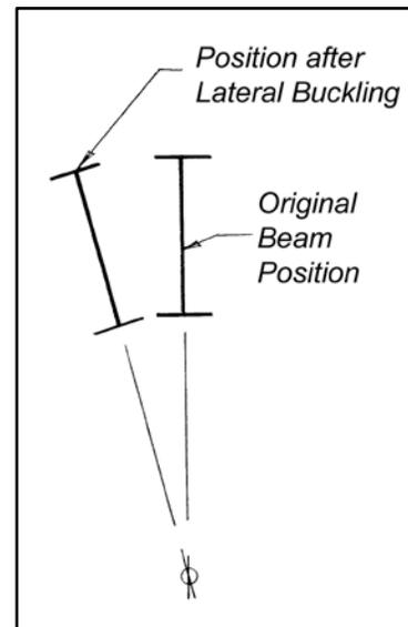
Figure 16 - Lateral buckling of top flange
