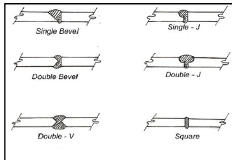
Figure 5- Butt Welds
