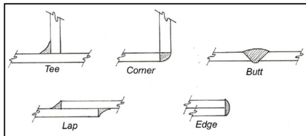
Figure 6 – Weld Joints
