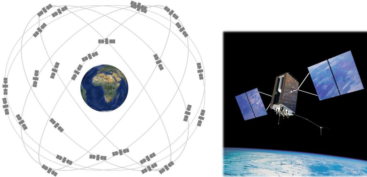
GPS constellation of satellites (left) & a modern satellite in orbit (right)
