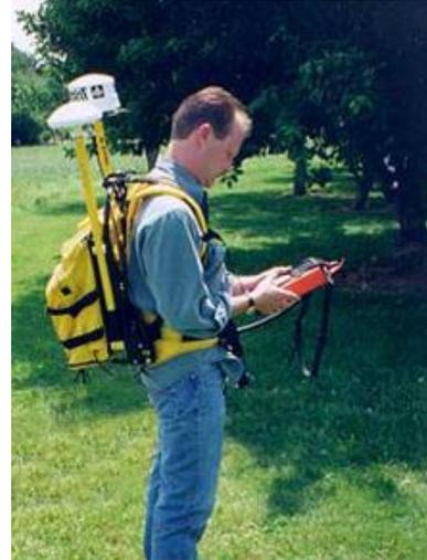
Backpack mounted GPS roving antenna and receiver unit
