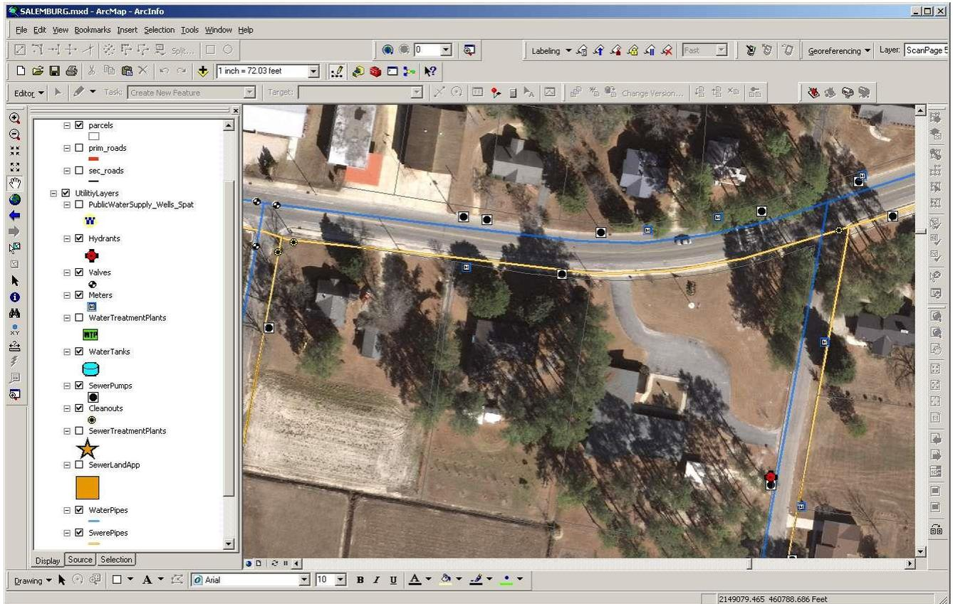
A utility map within a GIS showing water and sewer lines, valves, sewer pumps, and fire hydrants
