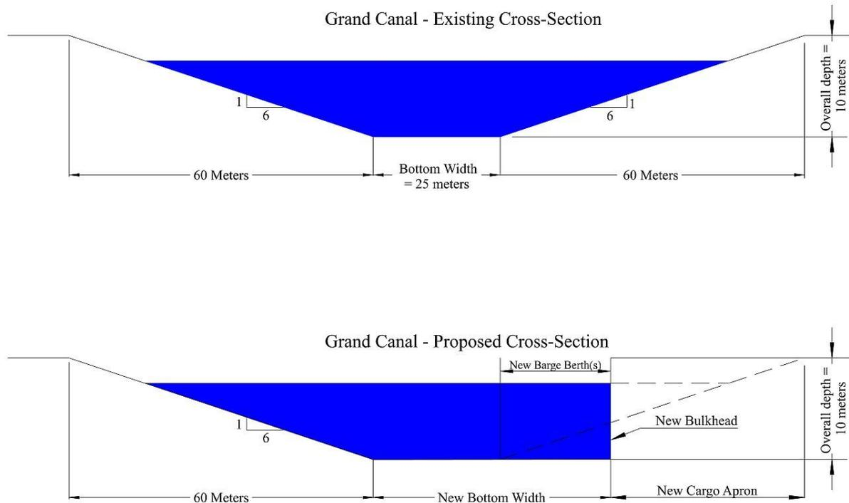
Figure 29 Existing and Proposed Cross-Section
