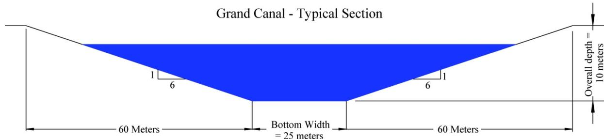
**Figure 26 Existing Cross-Section**
