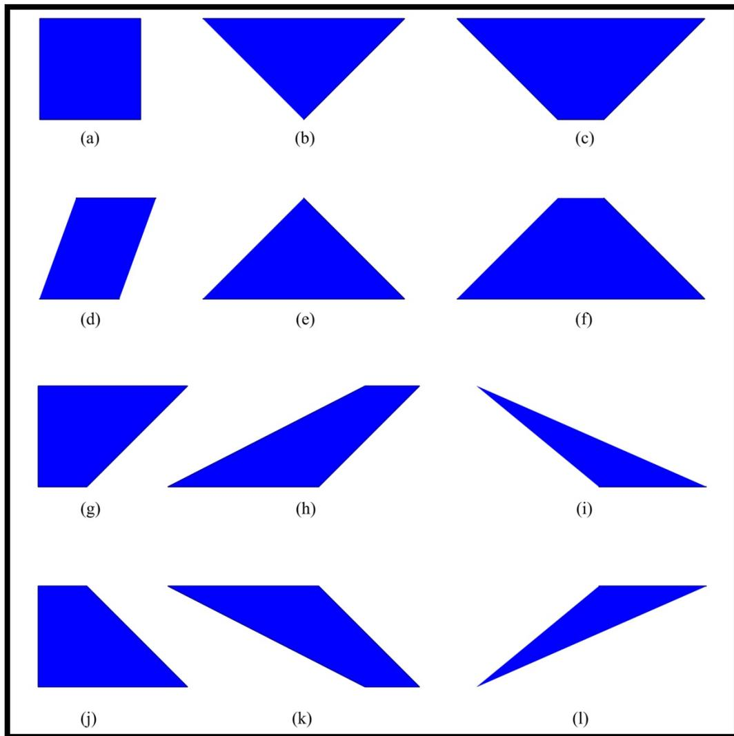
Figure 18 - Manning-Channel allowable shapes
