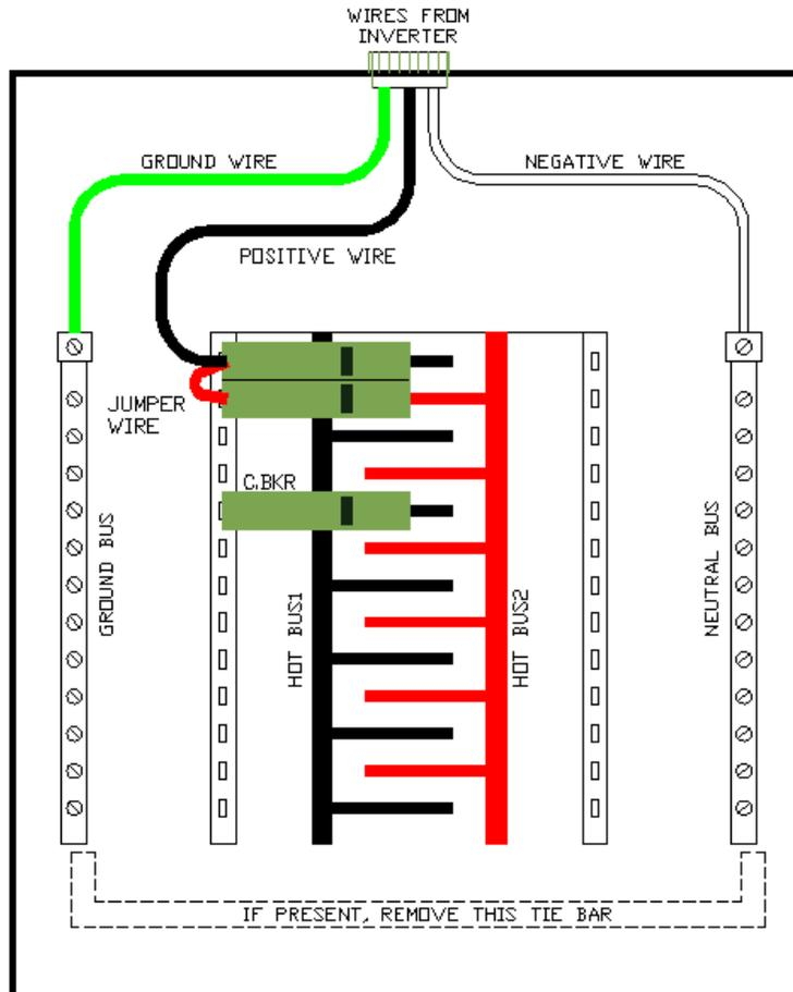
*Circuit Breaker Box wiring using circuit breakers to feed both Hot Bus bars*
