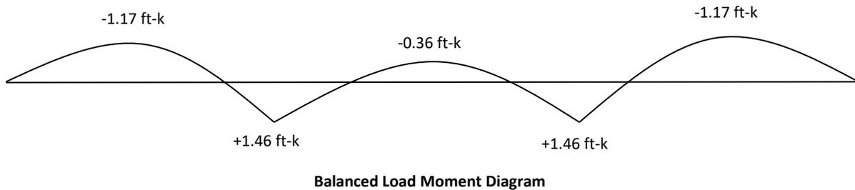
Note that the balanced load due to the tendon is acting upward, and hence the moments are in the opposite direction of the gravity load moments.
