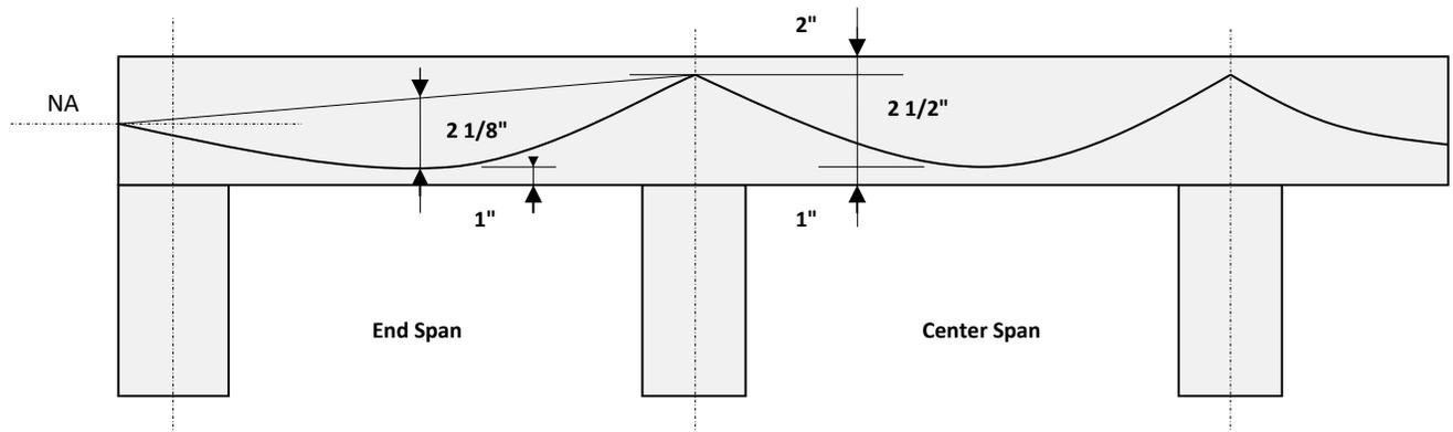
Next, we will determine the effective post-tensioning force required to balance 65% of the dead load, or 45 psf. Recall from Part One of this course that the effective post-tensioning force,  $F_e$ , is the force in the tendons after all losses and is computed as:
