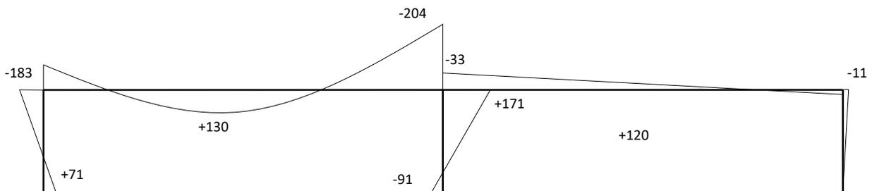
Live Load Moments – Left Span Loaded (ft-kips)
