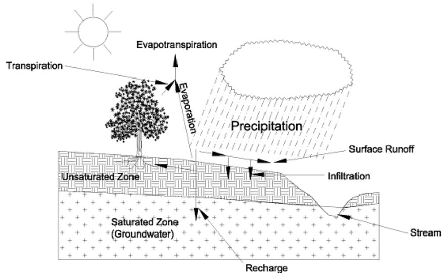
**Schematic Showing Groundwater Recharge in the Hydrologic Cycle**
