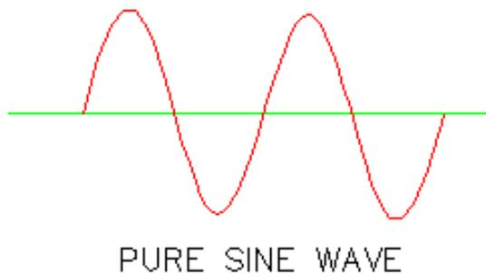
Ideally, you want the inverter to produce power that replicates this wave as closely as possible for our use in the structure to avoid problems.
