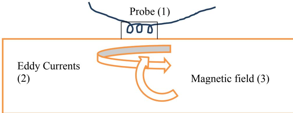
Alternating magnetic field from the probe (1) induces eddy currents (2) within the part. These eddy currents induce their own magnetic field (3) within the part creating measurable impedance in the probe (1)
