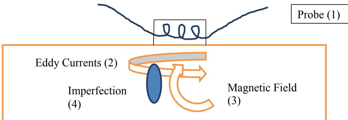
An imperfection (4) alters the eddy currents (2) and magnetic field (3) changing the measurable impedance created in the probe (1). Changes in the measurable impedance would also be caused by distance of the probe from the material, material composition, grain size, heat treatment condition, etc.
