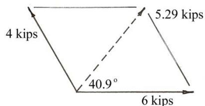
The **second** procedure, which we will use in this course, requires as a first step, that the two forces be resolved into their horizontal and vertical components. Then, the horizontal components are added to find a single resultant horizontal force, and the vertical components are added to find a single resultant vertical force. The problem is then one of finding the resultant of two orthogonal forces.
