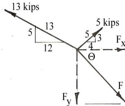
First determine the magnitude of the horizontal component and the magnitude of the vertical component of the unknown force. Note: because the forces are in equilibrium, the unknown force is equal in magnitude and opposite in direction to the resultant of the other forces.
