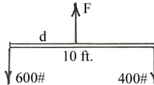
First determine the magnitude of the unknown force by summing forces vertically using the tally method.
