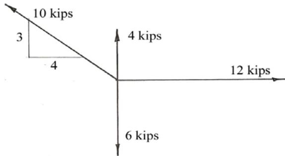
The slope or direction of a force is often stated by specifying the horizontal and vertical relationship – in this case 3 and 4. The hypotenuse of this triangle is 5. It is a 3-4-5 triangle. Another common one is the 5-12-13 triangle. Notice that 10k is twice 5. Therefore, the vertical component is twice 3, or 6 kips; and the horizontal component is twice 4, or 8 kips.
