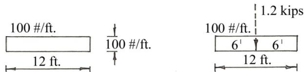
$$\begin{aligned} R &= (12 \text{ ft.}) (100 \text{ #/ft.}) = 1,200 \text{ #} = 1.2 \text{ kips} \\ x &= (1/2) (12 \text{ ft.}) = 6' \text{ from each end} \end{aligned}$$
