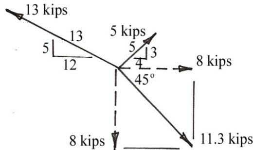
**Two Unknown Forces** If the two unknowns of a concurrent force system are the magnitude of two forces, you must write two equations, each equation summing the forces in a different direction. Usually the directions are horizontal and vertical (but they can be any direction). If each of the unknowns appears in each equation, the equations must be solved simultaneously. However, in some problems the equations can be written so that they are independent and can be solved independently.
