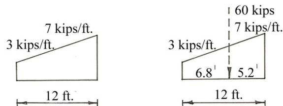
that is slightly more difficult, and requires a bit more thinking than breaking the load into two components. Using two components is the simplest way to do it and is the preferred way - there is less chance to make an error using the real simple math for two resultants. Shown below is the “answer” for replacing the trapezoidal load with only one resultant.
