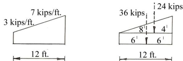
There is an alternate solution to the trapezoidal load. Instead of replacing the trapezoidal load with two resultants, replace the entire trapezoidal shape with only one resultant. The math to do
