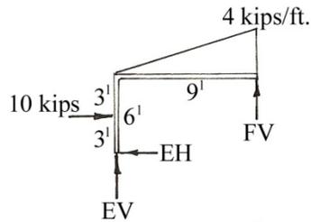
Begin by finding the resultant of the triangular load. The resultant has a magnitude equal to the area under the load diagram; is located at the centroid of the load diagram, which is at the two-thirds point; is parallel to the load diagram; and is shown as a dashed line.
