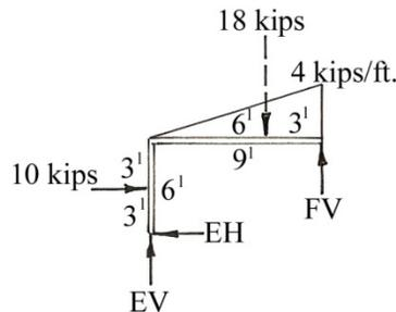
Since there is only one unknown in the horizontal direction, begin by summing the forces horizontal equals zero to determine EH
