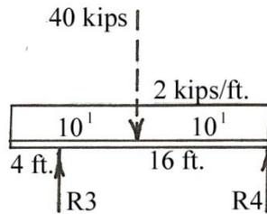
First determine one equilibrium equation by summing forces vertically using the tally method.
