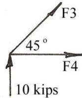
Since the final directions of forces F3 and F4 may not be obvious, it is convenient to “guess” their direction as tension as shown above before beginning the solution for their values. If the solution for either, or both, produces a negative value, it simply means that the assumed direction was not the correct direction.
