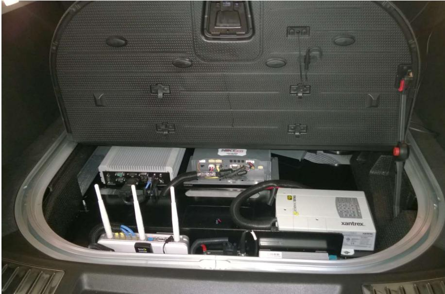
Figure 15. FHWA connected vehicle on-board equipment
