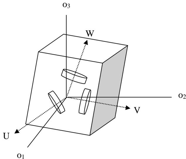
**Figure 3.15: Momentum Transfer – Reaction Wheel Configuration**
