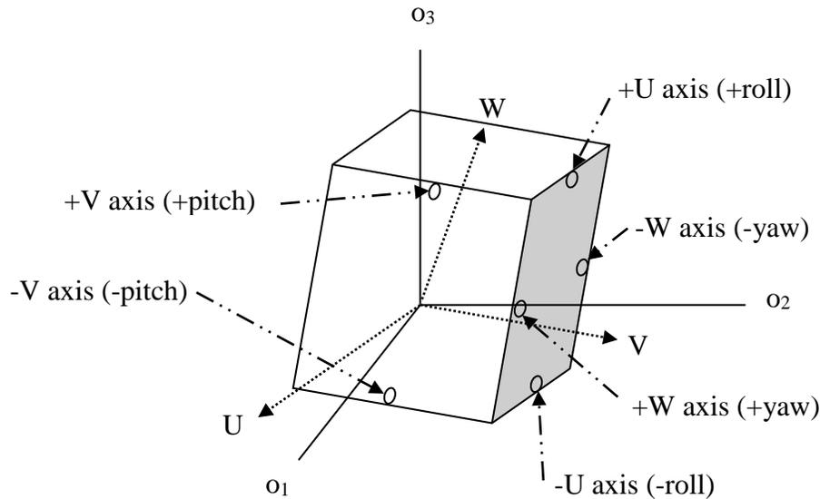
**Figure 3.14: Mass Expulsion – Thrust Nozzle Configuration**
