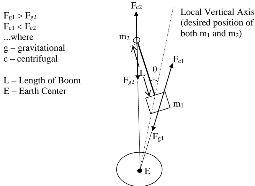
**Figure 3.12: Gravity Gradient Forces**
