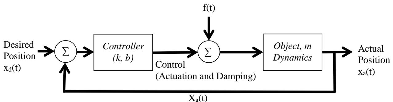
Figure 3.5: Mass-Spring-Damper Control System
