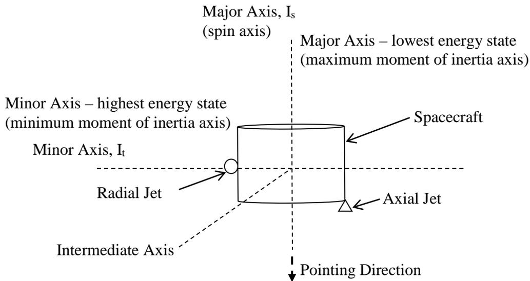
**Figure 3.8: Body Spin Control Method**
