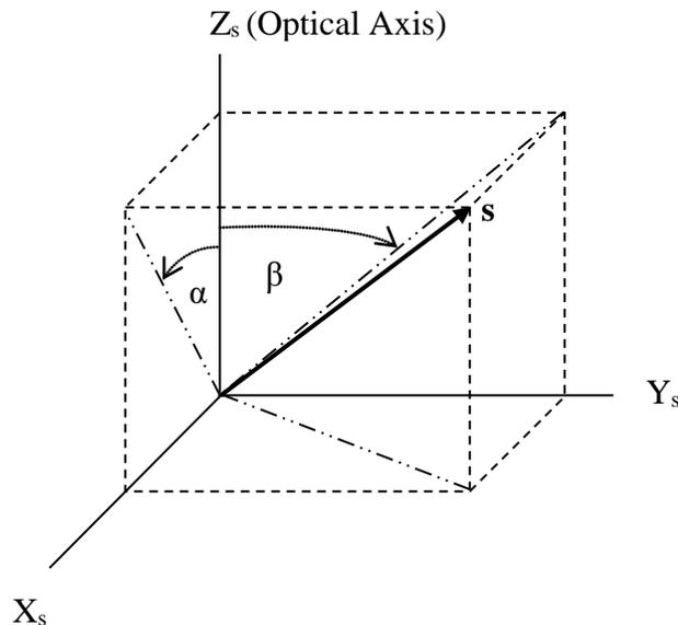
**Figure 2.4: Sensor Coordinate System – Sun or Star**
