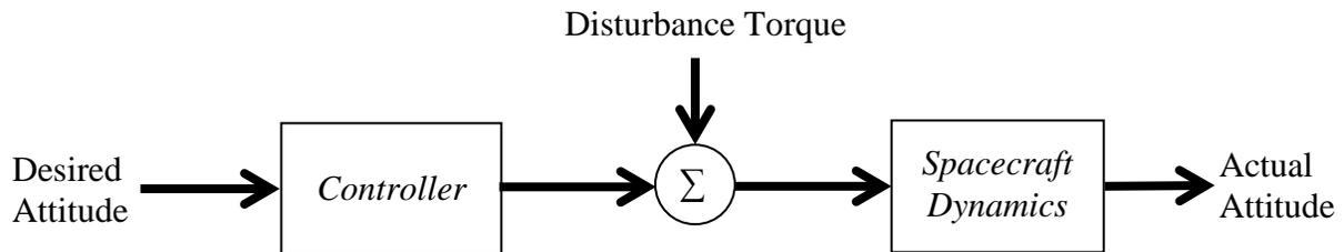
**Figure 3.6: Open Loop Control System**
