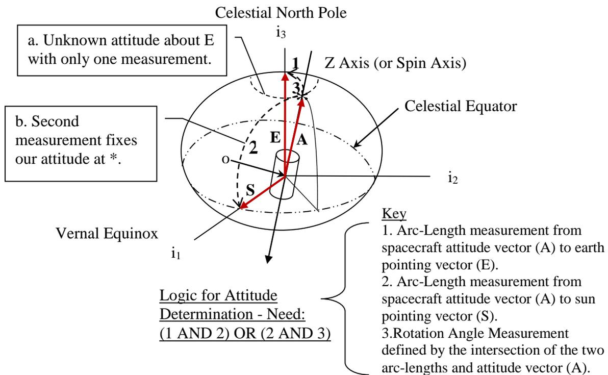
Figure 2.9: Single-Axis Attitude Measurements
