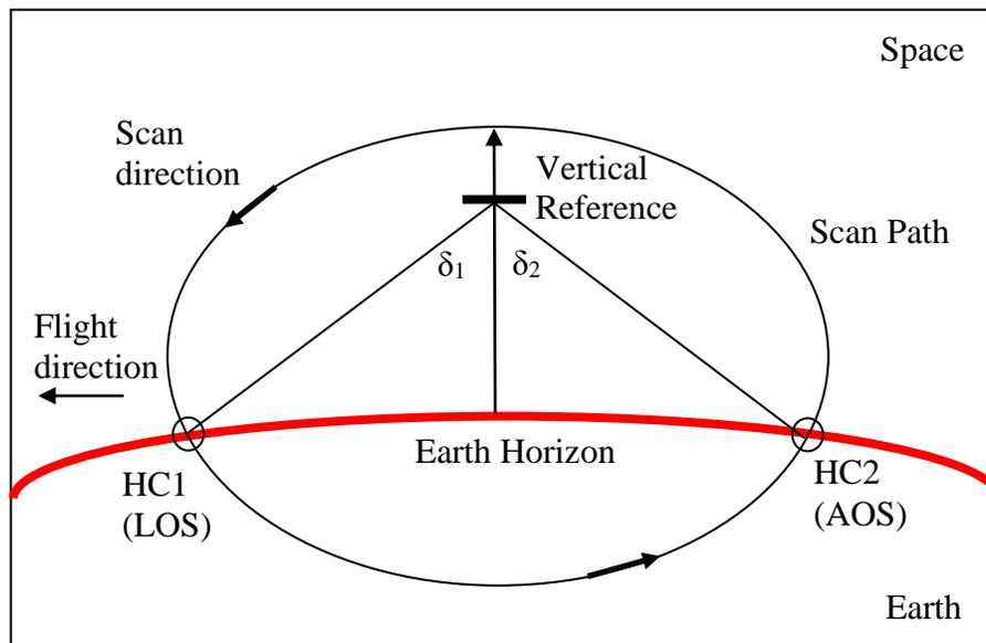
**Figure 2.7: Earth Scanning Horizon Sensor**
