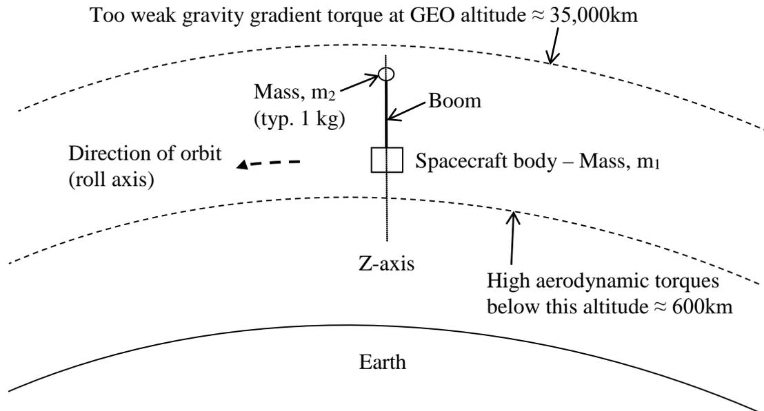
**Figure 3.11: Gravity Gradient Control Method**
