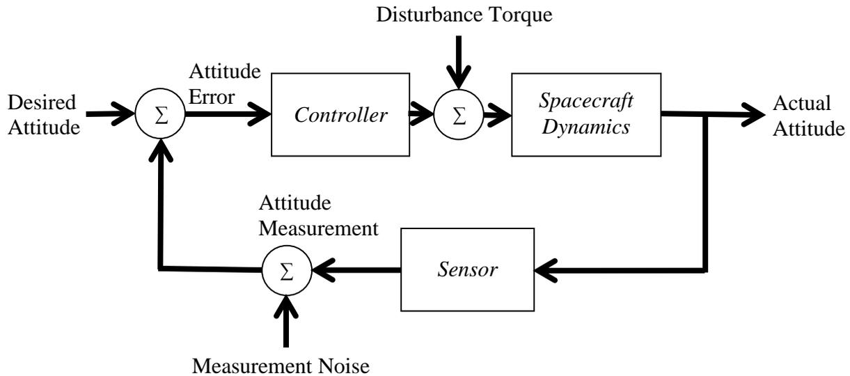
Figure 3.7: Closed Loop Control System
