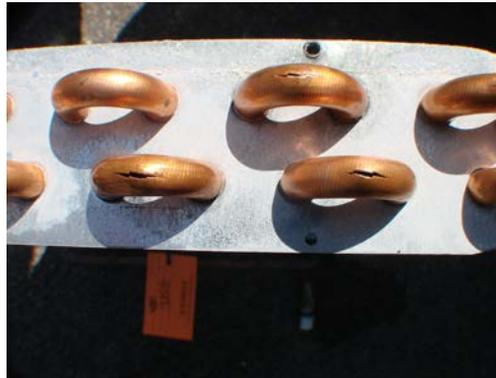
Here is a heater coil failure with close-up photo from an SLR and even closer from a USB microscope on its low 40x setting. The USB can do 400x as well but I find the 40x really useful for detailed evaluations, and leave the 400x to the metallurgist. This is a freezing case.
