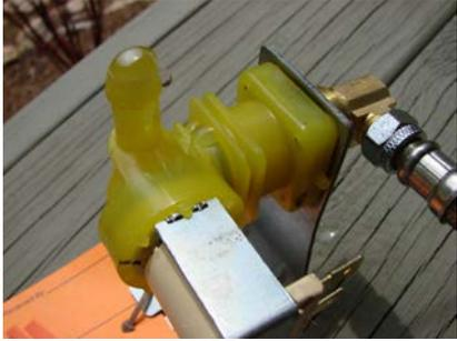
This is a dishwasher inlet valve being tested under water pressure only, no power applied. Water leaks past the seat, and this is likely due to a manufacturing defect. The valve should be opened and inspected to demonstrate the defect, but that would be a destructive test and should wait for a joint inspection.
