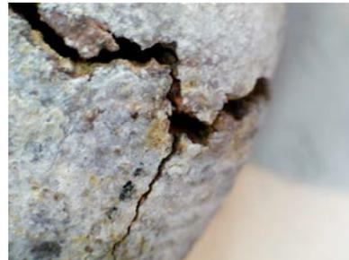
A close photo of a failed valve body. This valve was sent to a metallurgist for materials analysis. Energy-dispersive X-ray spectroscopy (EDS), shown below, determined that the failure was the result of dezincification. This is a manufacturing defect.
