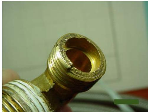
This case arose from a document and evidence review. The fitting failed across the threads at a flexible hose connection, which doesn't put much bending stress on the nozzle. The material was sent to a metallurgist who determined that the cause was stress corrosion cracking.
