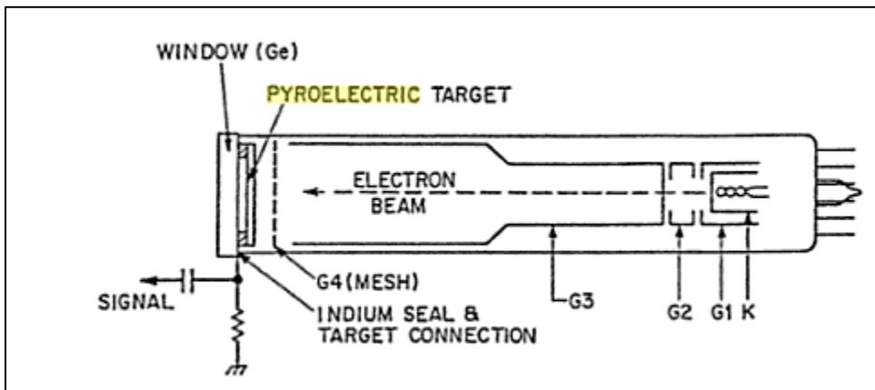
**Pyroelectric vidicon (PEV) tube**
