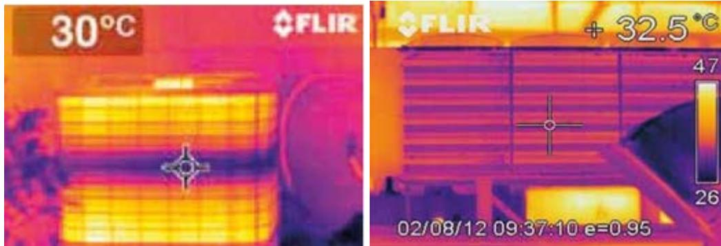
The image is of a blocked HVAC unit as compared to an unblocked unit. The bright color reports the higher temperature of the blocked unit. The equipment is overheating and operating above the normal temperature. By detecting the blockage early, the equipment can be repaired before it fails and is damaged.
