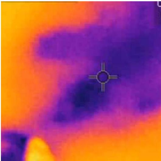
A change in temperature of the ceiling surface is indicated by the dark image in the photograph. The thermal camera was used to perform an initial assessment of the ceiling. The suspicious image was examined with a moisture meter which confirmed the presence of water damage caused by a low spot on the roof.
