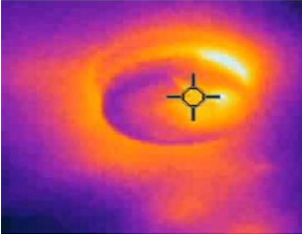
A change in temperature of the ceiling surface is indicated by the bright image in the photograph. The thermal camera was used in to examine the ceiling penetration. The image indicates a loss of energy through the ceiling, which was confirmed by seeing missing insulation in the attic.
