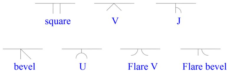
**Figure 13** Basic groove weld symbols (arrow side shown)
