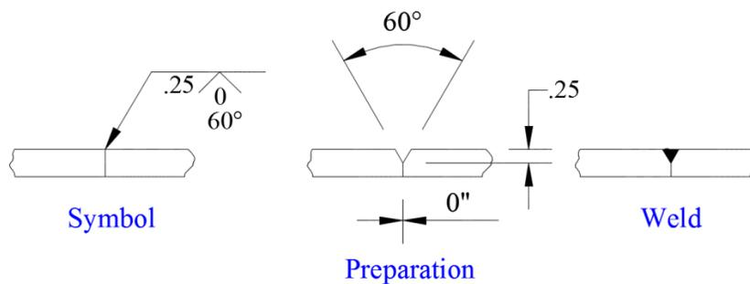
**Figure 16** Partial penetration (or partial depth) V-groove weld
