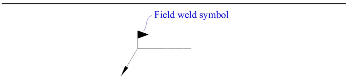
**Figure 5** Field weld symbol
