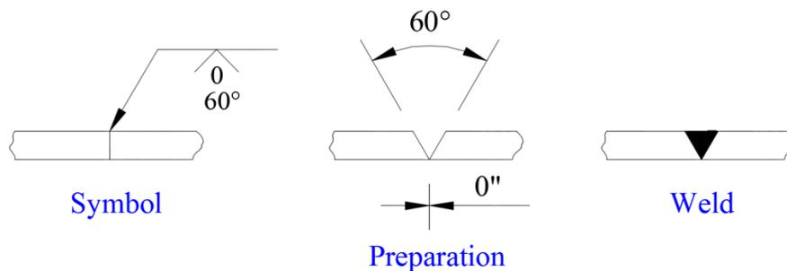
**Figure 14** Full depth V-groove weld (one side)
