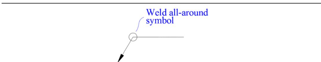
**Figure 6** Weld all-around symbol
