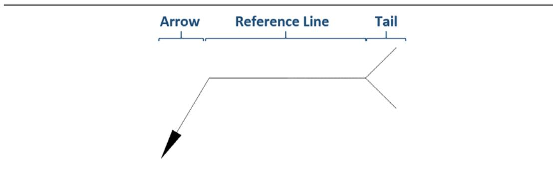
**Figure 2** Basic components of a welding symbol
