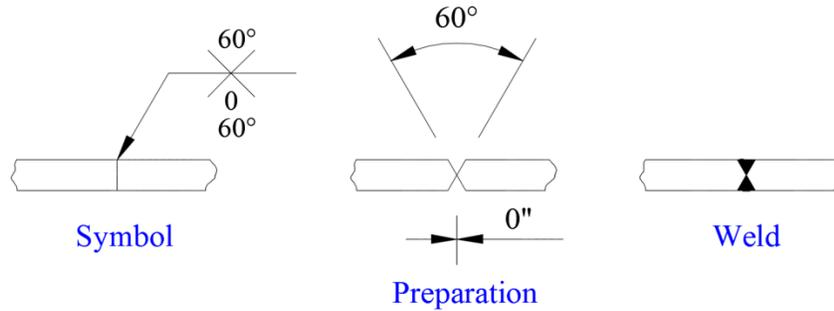
**Figure 15** Full depth V-groove weld (both sides)
