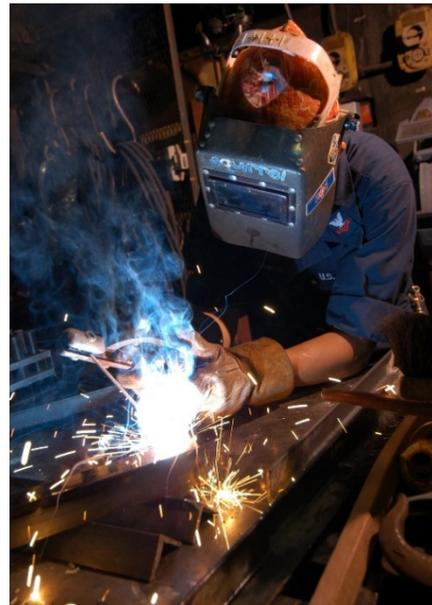
**Figure 1** Arc welding
