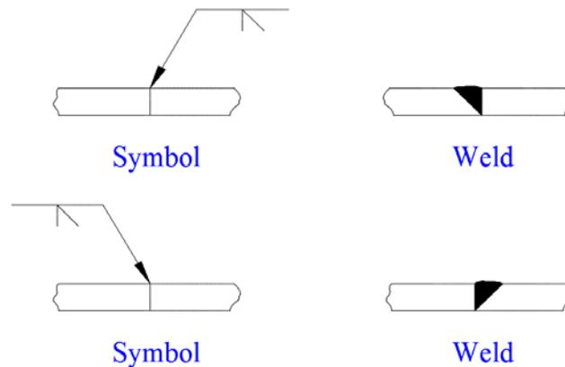
**Figure 17** Bevel weld for butt joints
