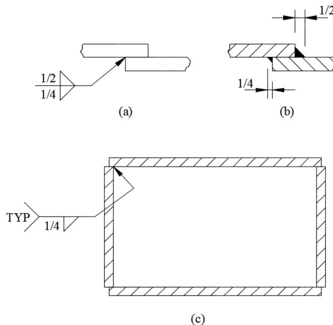
**Figure 9** Fillet weld size examples (a) weld symbol (b) resulting weld (c) usage of welding tail and typical callout for multiple welds
