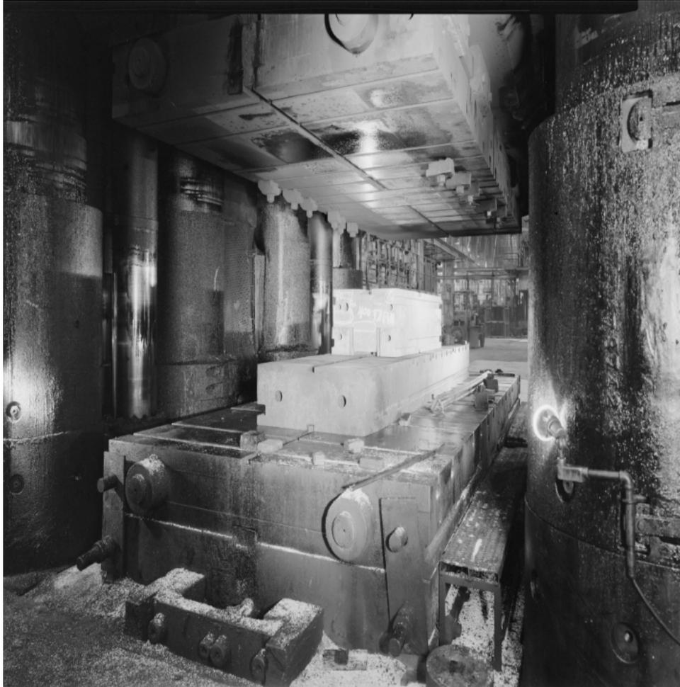
*Figure 11* Alcoa Forging Division 50,000-ton closed die forging press
