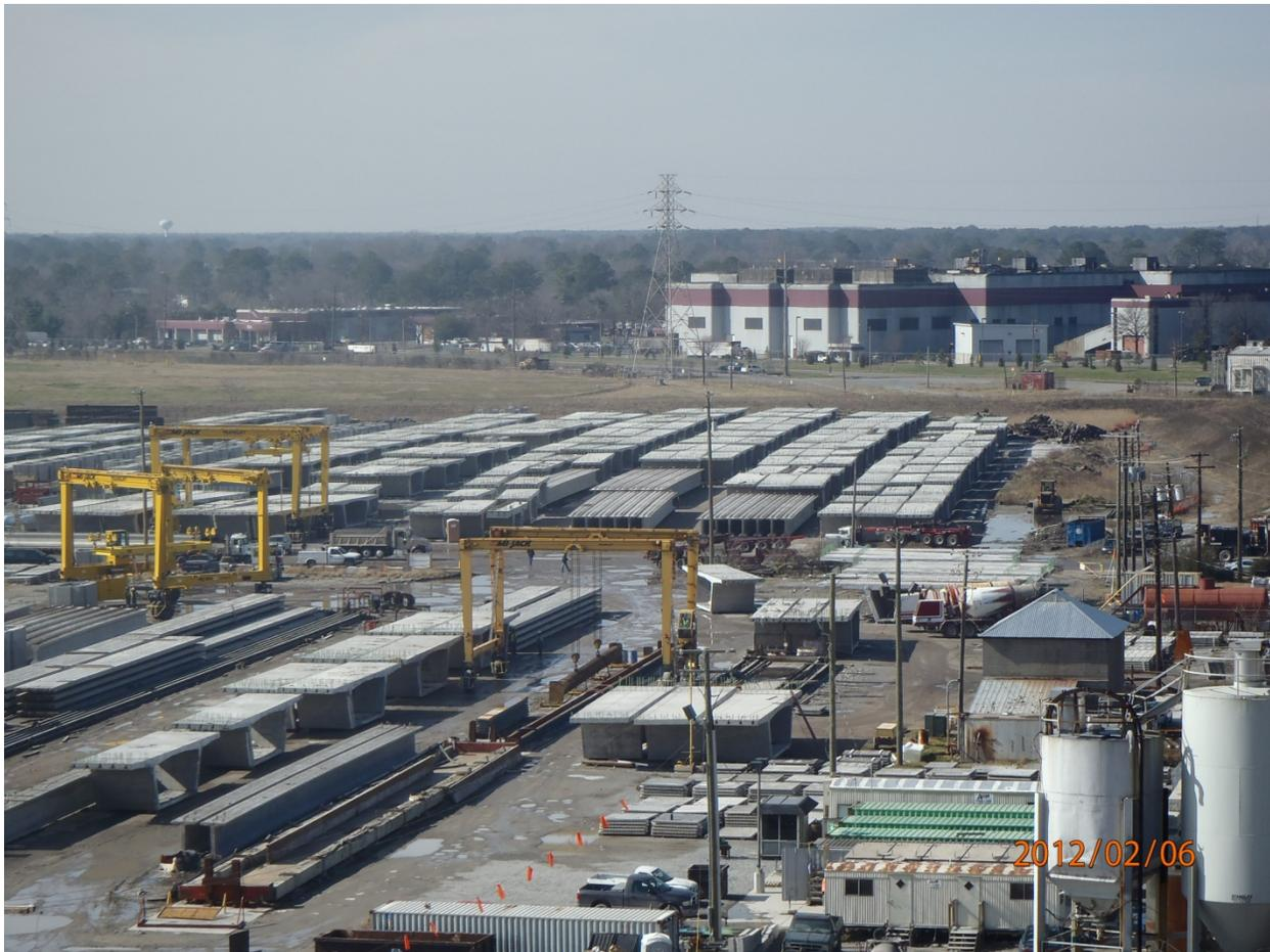
After a day's production, the previous day's match cast segment is ready to be finished and set for storage. Depending on the design, some segments can be lifted and placed in storage prior to any post-tensioning. This will be a factor of strength gained during
