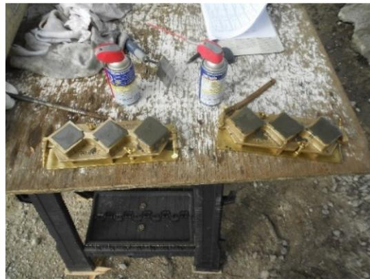
Grout cubes and flow tests are performed by the QC department to ensure the grout meets the specifications and the operations are acceptable.
