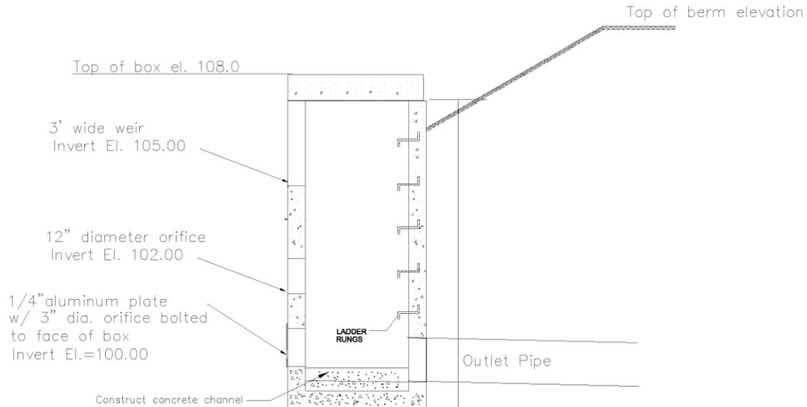
Outlet Structure Detail: Side View
