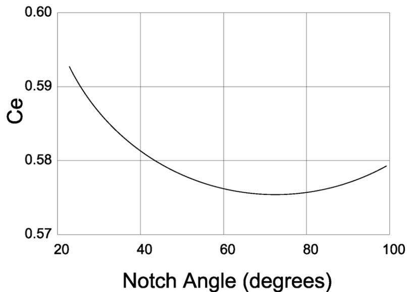
$X$  is the angle of the notch in degrees
