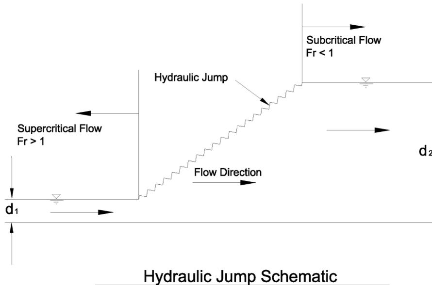
The basic formula governing the geometry of a hydraulic jump is shown below:
