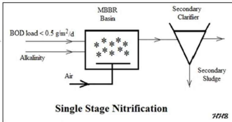
**Figure 8.** Single Stage MBBR Process for Nitrification
