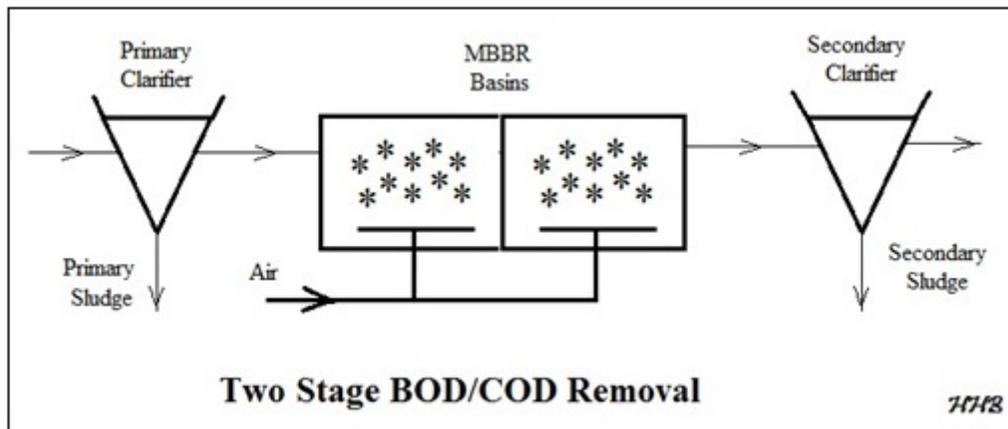
**Figure 12.** Two-Stage MBBR Process for BOD/COD Removal
