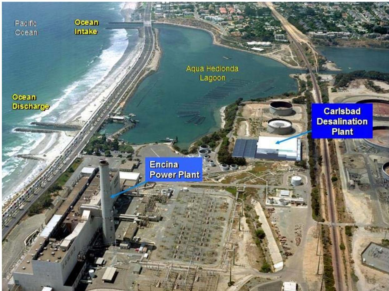
**Figure 11 – Configuration of Intake and Discharge of Carlsbad Desalination Plant**
