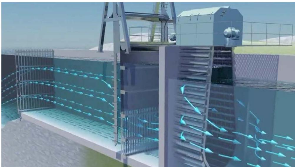
**Figure 2 – Intake Coarse Screen followed by Fine Screen**
