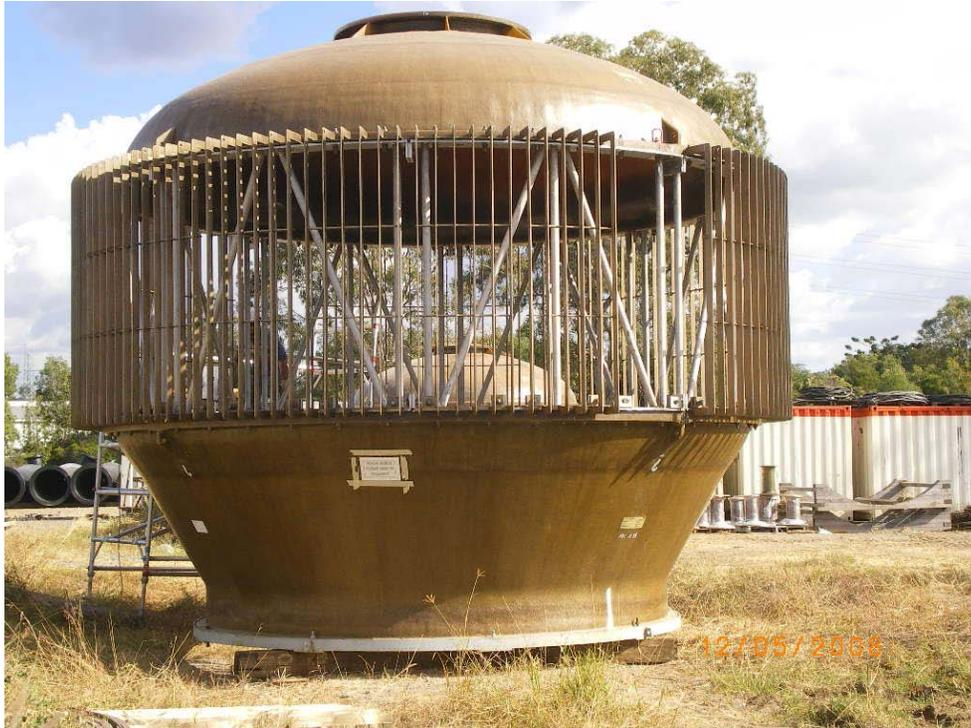
**Figure 1 – Intake Bar Screen**
