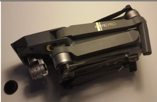
*Folded drone with sun filter removed. Round Downward sensors are visible. Transparent plastic gimbal clamp & camera cover are off in the picture to the right.*
