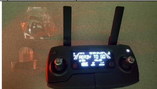
*Push the Left stick forward and the drone will rise. Toward pilot and drone descends. Push Left or Right to rotate (yaw turn) the drone. Right stick forward and drone advances forward. Toward pilot and drone backs up. Left or Right for drone to fly left or right.*
