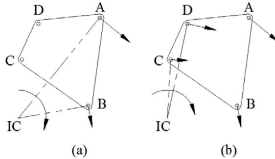
Figure 12 (a) Locating the instant center of rotation (b) Determining velocity of points using the instant center (Doane, 2015) [reused with permission]
