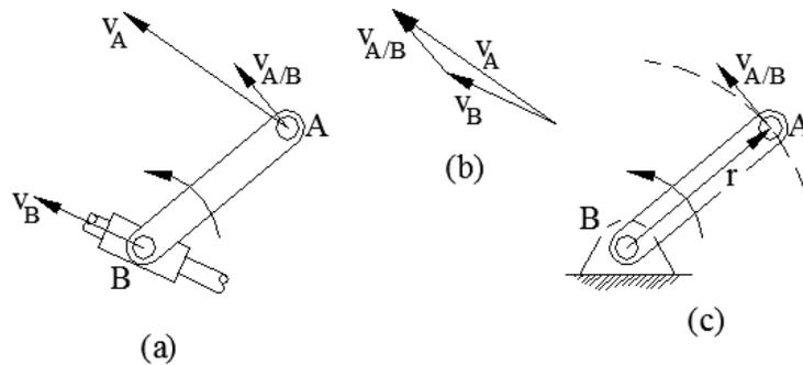
Figure 11 (a) Velocity difference (b) Vector polygon (c) Representation of the velocity of point A with respect to point B (Doane, 2015) [reused with permission]
