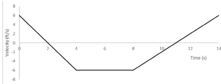
The acceleration becomes  $2 \text{ ft/s}^2$  at a time of 8 seconds, and it remains constant until 14 seconds. Using graphical integration, the change in velocity will equal the area under the curve. The velocity at 14 seconds will be
