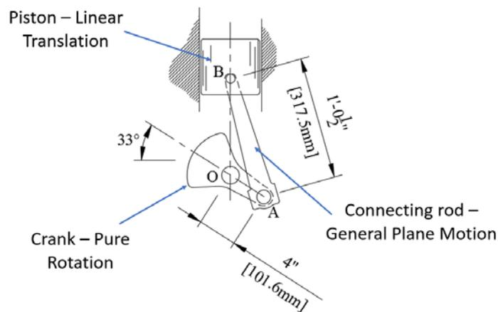
Figure 13 Component motions in a slider-crank mechanism
