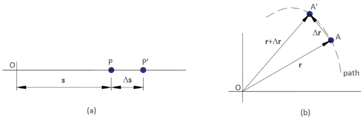
Figure 2 (a) Rectilinear motion and (b) Curvilinear motion
