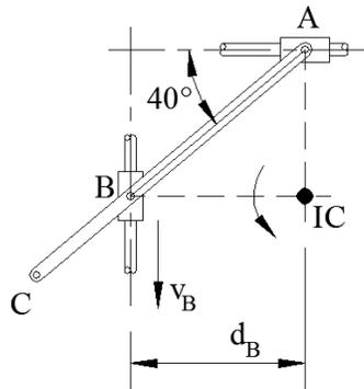
The distance from B to the instant center is required to determine the angular velocity of the rod.
