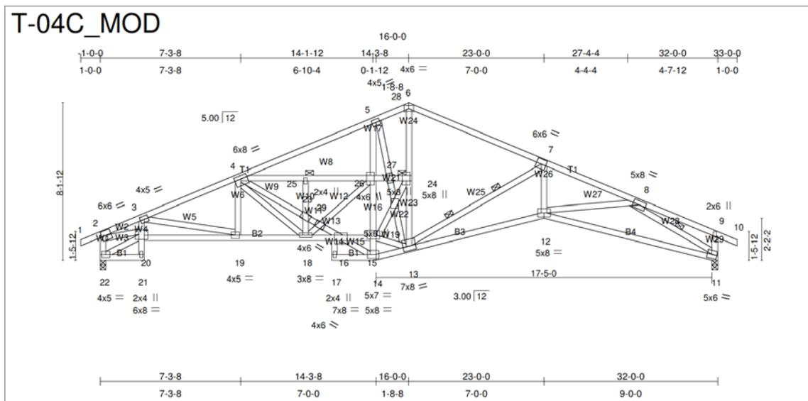
The second step in the Truss Model Method is to remove the members of the original truss leaving only what needs to be fabricated as the new scab truss. Once the members are removed, the final step is to manually change the plate sizes back so that the scab truss members have similar coverage on the scab truss as is shown in the composite design T-04C\_MOD shown above. The following photograph shows the completed repair.
