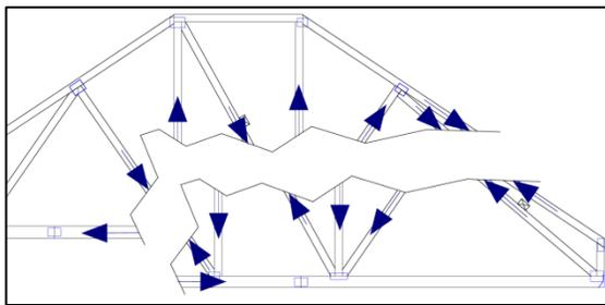
The Truss Sections Method effectively divides the original truss in two pieces or sections with the dividing lines being the perimeter of the scab truss. A free body diagram can be developed showing forces in each of the members along the split as shown in the diagram to the left. The key concept with the Truss Sections method is that some of these forces are applied to the scab truss
