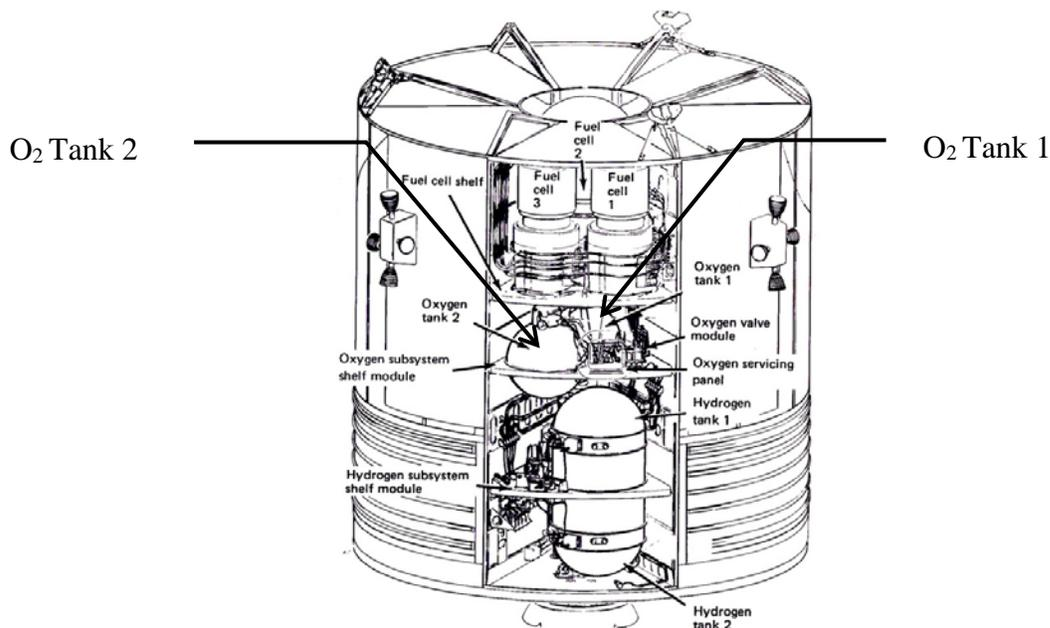
**Figure 1.1: Apollo Oxygen Tanks**
