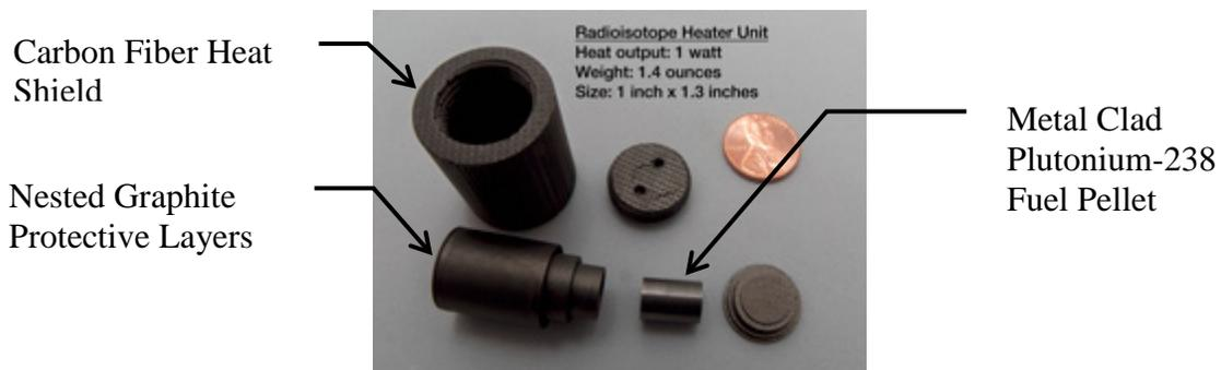
**Figure 3.1: Radioisotope Heater Unit**
