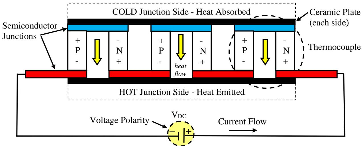
**Figure 3.2: Single Stage Thermoelectric Cooler**
