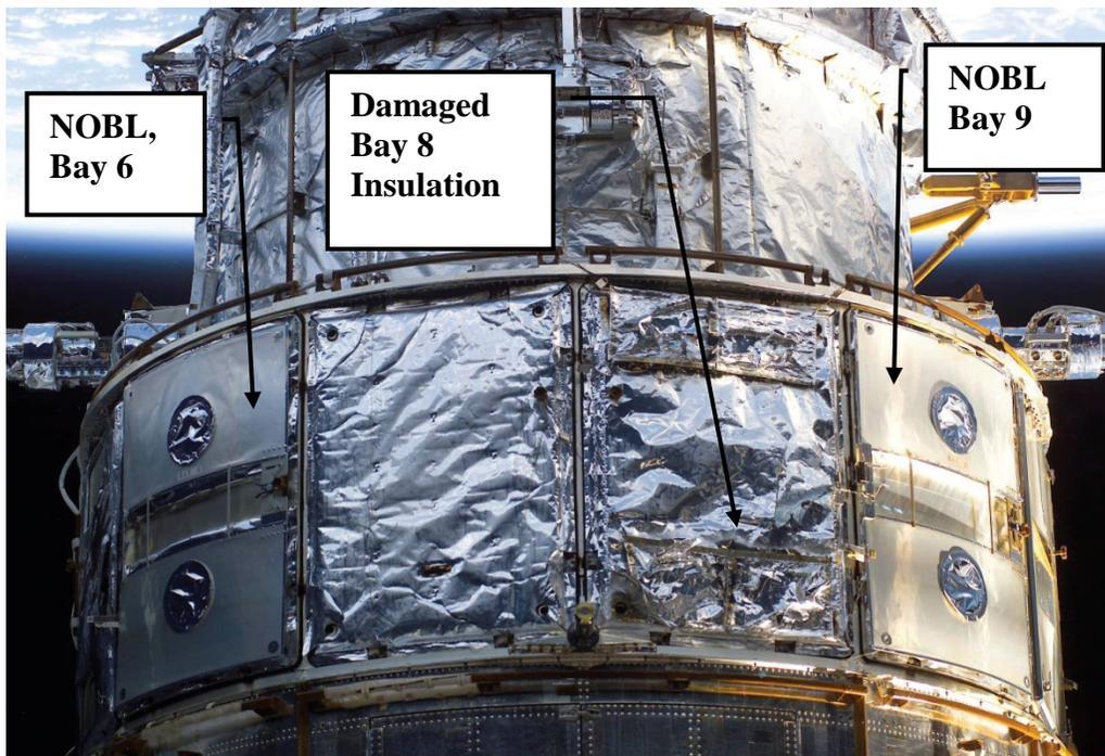
**Figure 2.4: Spacecraft Hubble - Thermal Insulation**
