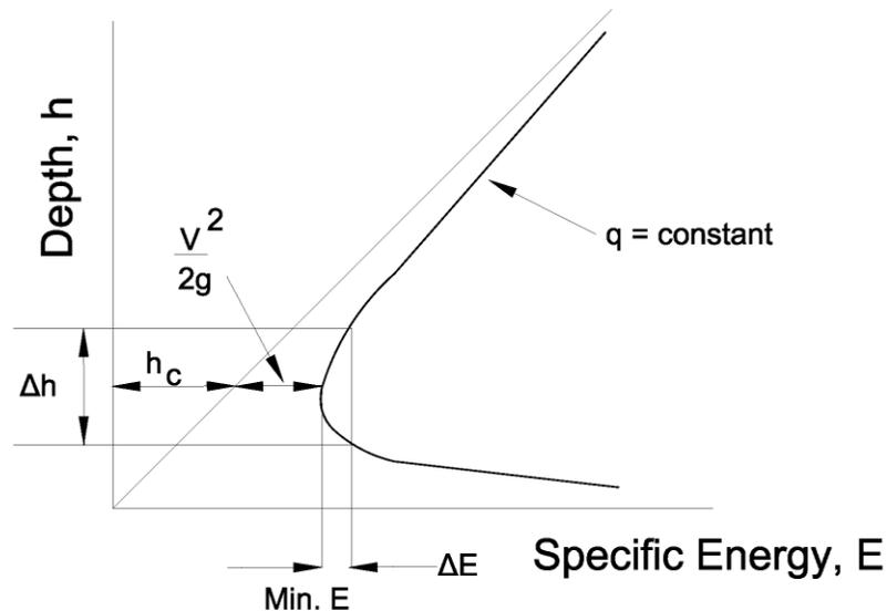
Specific Energy Curve for Open Channel Flow
