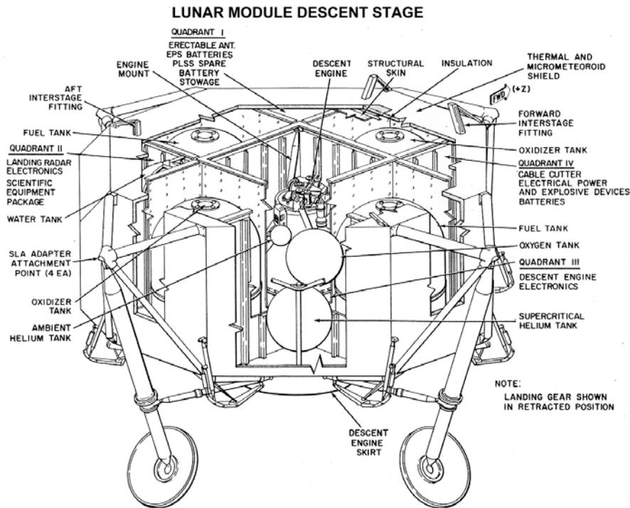
**Figure 1.4: Apollo Lunar Module Descent Stage Detail**
