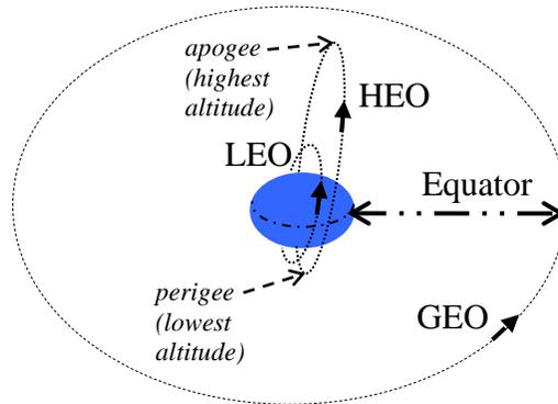
**Figure 1.1: Common Earth Orbit Types**
