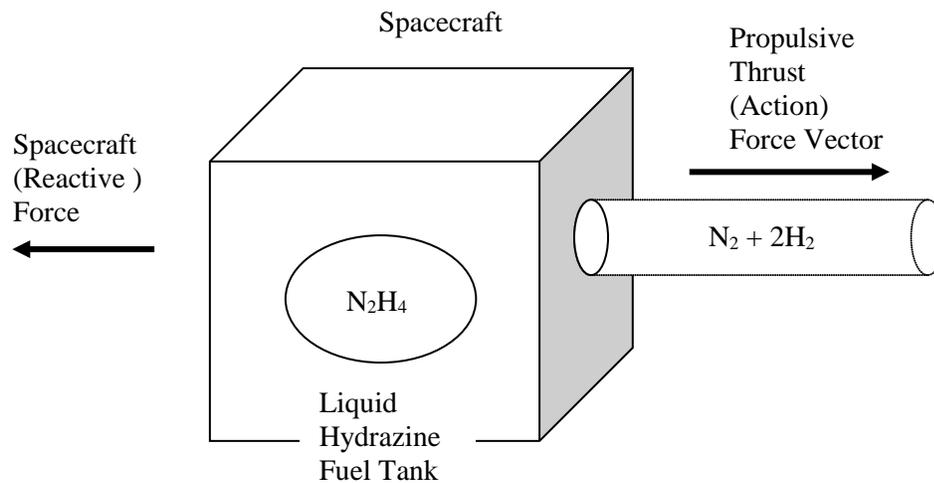
**Figure 2.1: Hydrazine Decomposition Reaction**
