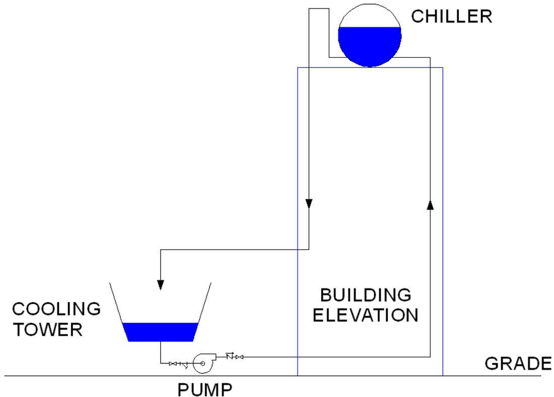
Figure 15: Condenser Water System – Problem Solved
