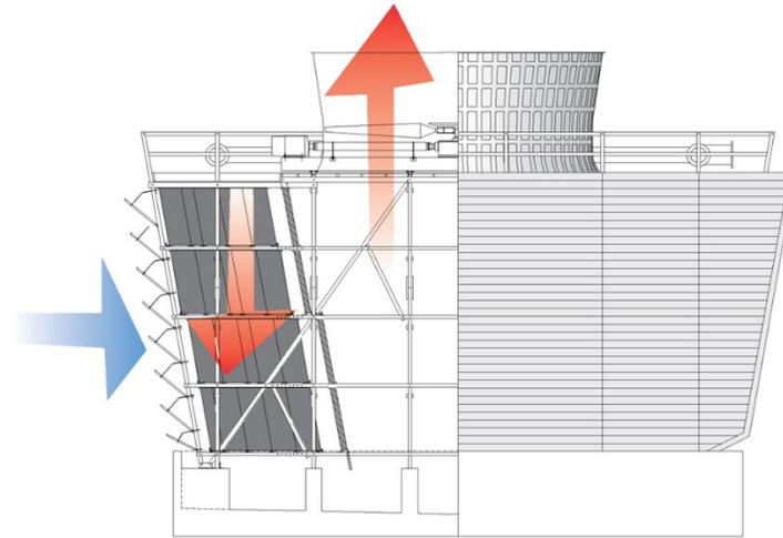
Figure 6: Crossflow Cooling Tower
