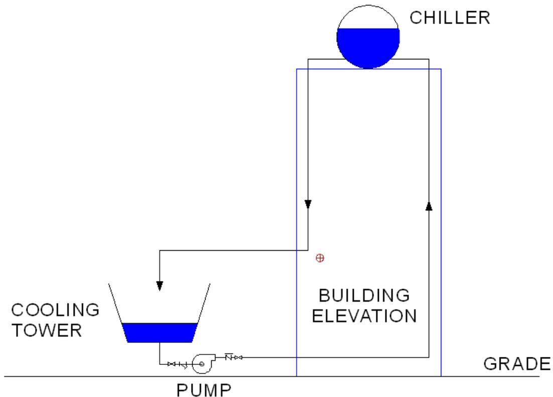
Figure 14: Condenser Water System
