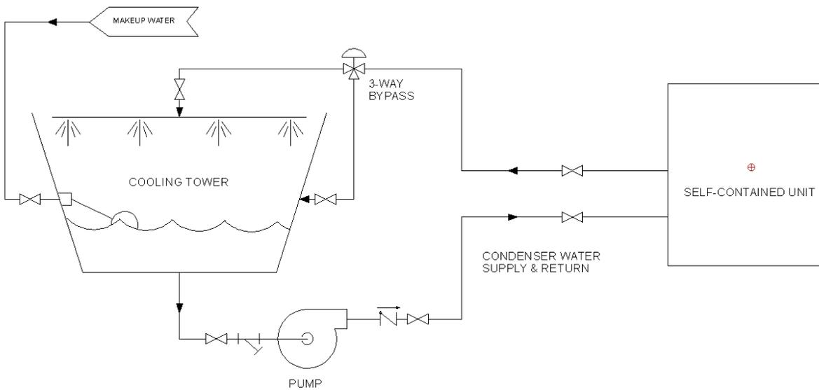
Figure 13: HVAC Cooling Tower Application: Self-Contained Unit
