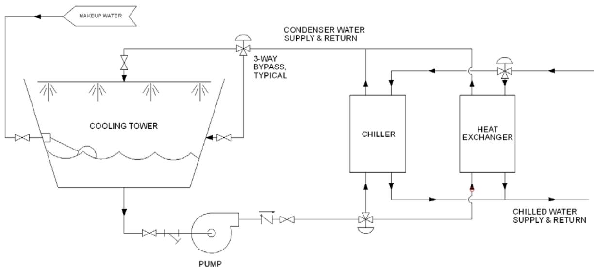
Figure 12: HVAC Cooling Tower Application: Free Cooling Arrangement
