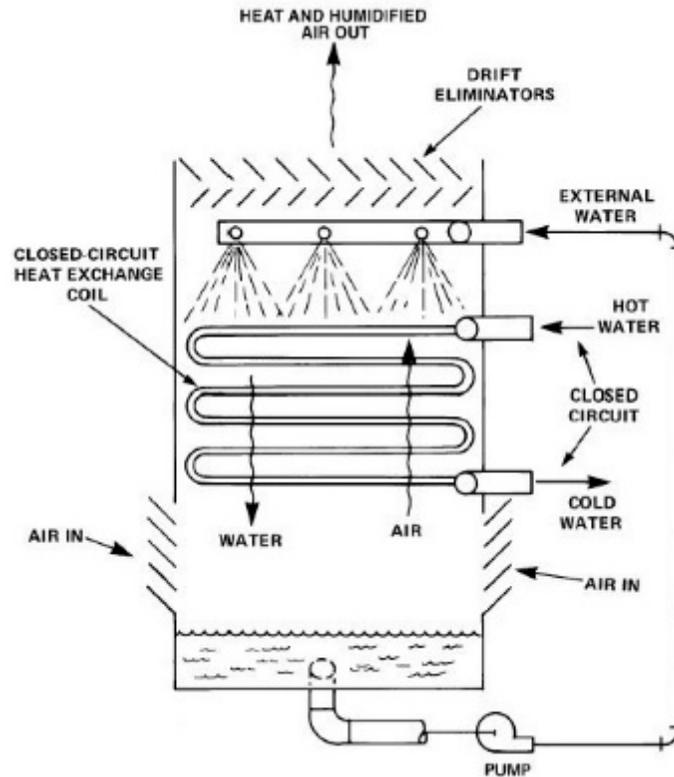
Figure 5: Indirect Cooling Tower Diagram
