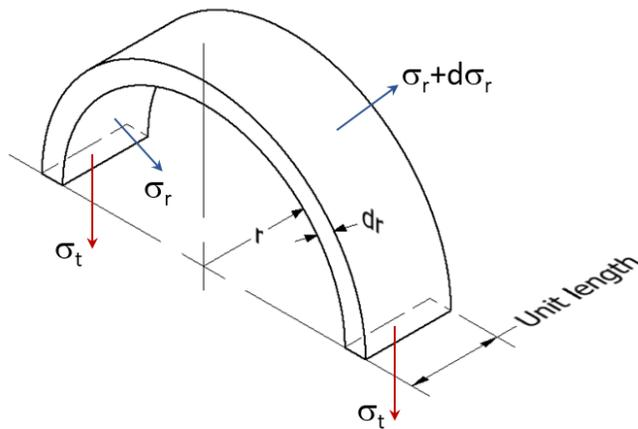
Figure 8 Stresses on the half shell
