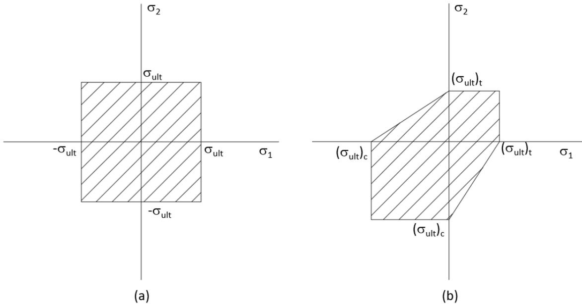
Figure 11 Brittle material theories (a) Maximum stress theory (b) Mohr's failure criterion
