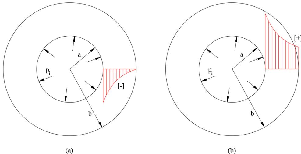
Figure 9 (a) Radial stress distribution and (b) tangential stress distribution for internal pressure only
