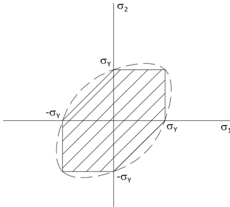
*Figure 12* Ductile material theories: Maximum shear theory (solid line shaded region) and Von Mises yield theory (dashed line)
