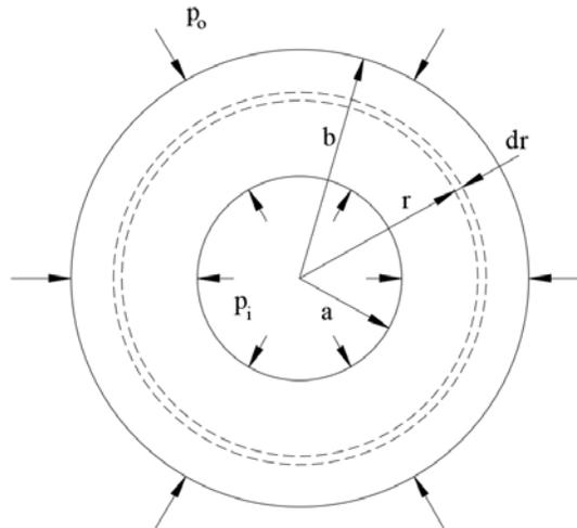
Figure 7 Internal and external pressure on a thick-walled cylinder
