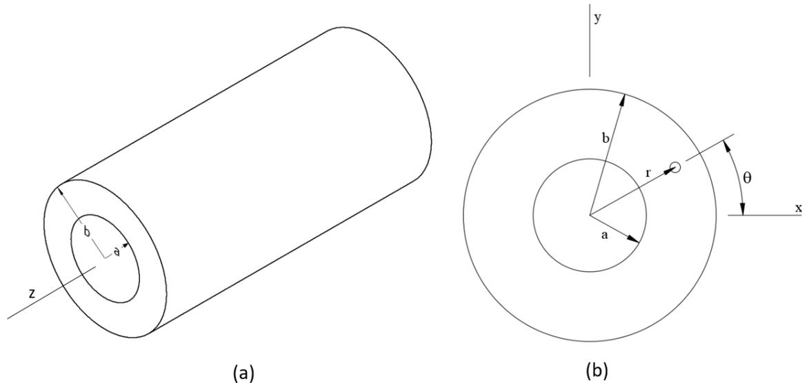
Figure 6 Thick walled pressure vessel and cylindrical coordinate system
