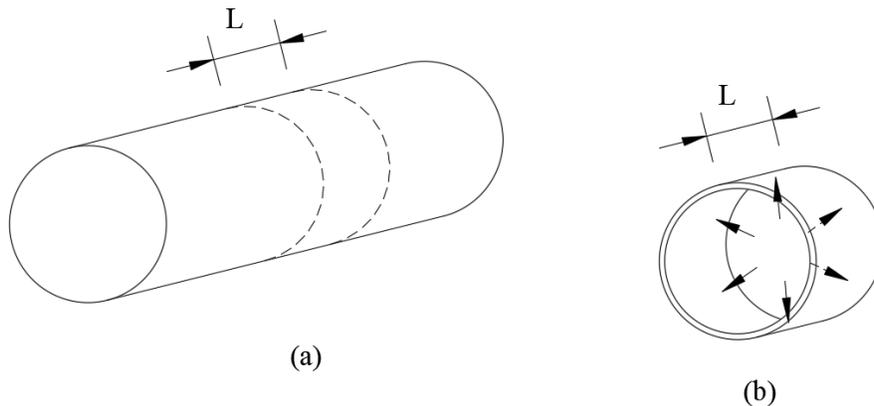
Figure 2 (a) Thin-walled pressure vessel (b) Isolated section
