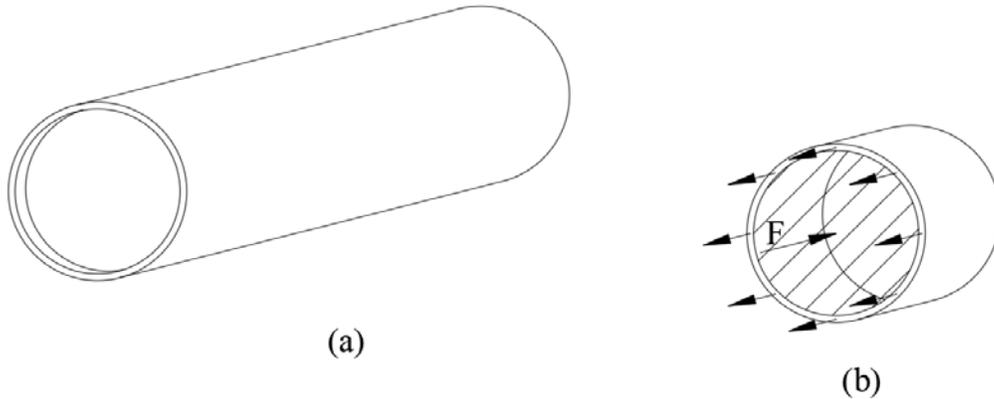
Figure 4 (a) Thin-walled pressure vessel with closed ends (b) Isolated section
