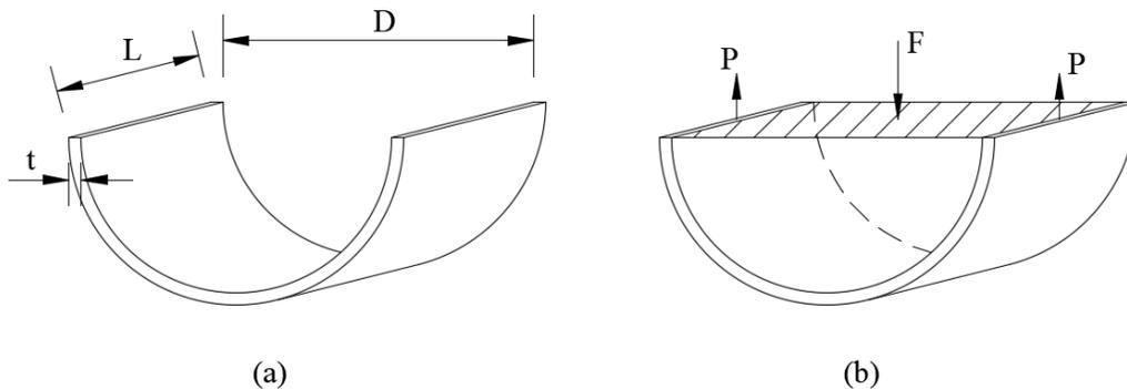
Figure 3 (a) Half section dimension (b) Forces on half section
