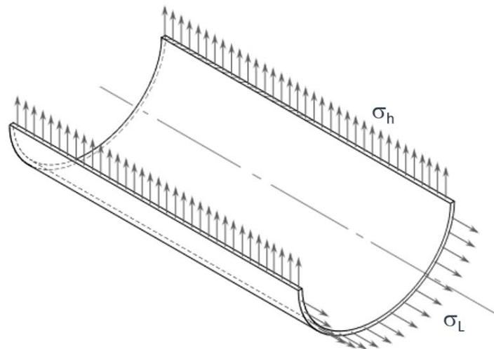
*Figure 1* Illustration of hoop stress  $\sigma_h$  and longitudinal stress  $\sigma_L$
