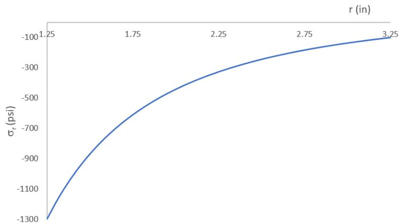
Note that the radial stress equals the internal pressure at  $a$  and the external pressure at  $b$  (all negative).
