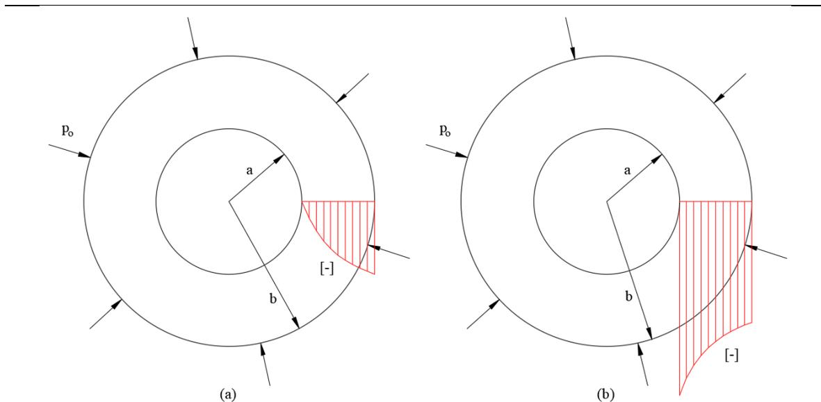
Figure 10 (a) Radial stress distribution and (b) tangential stress distribution for external pressure only
