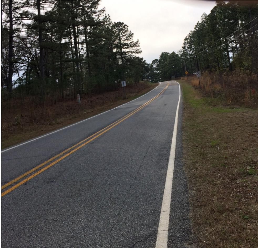
**Figure 4. Example of limited sight distance.**
