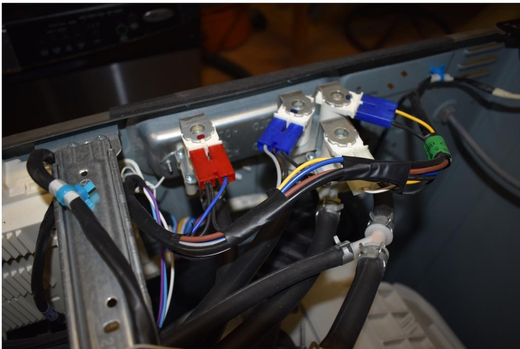
Photo #52 – This machine has four inlet valves. One is hot water and the others are cold water run through different sections of the detergent dispenser.
