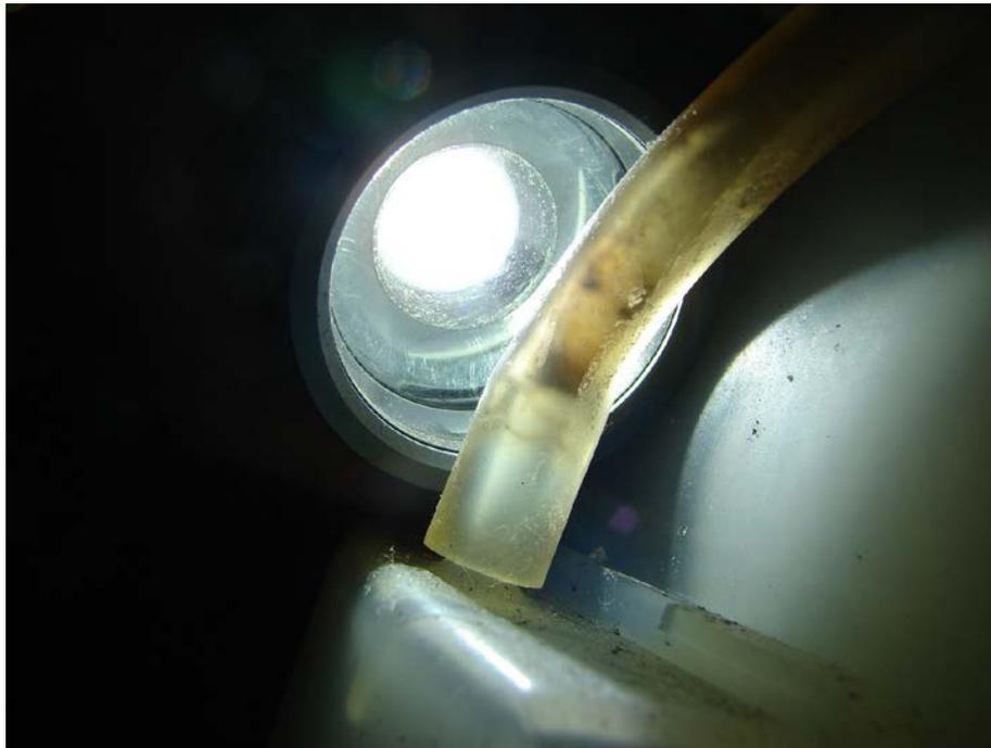
Photo #64 – Another case of blockage of the air tube.
