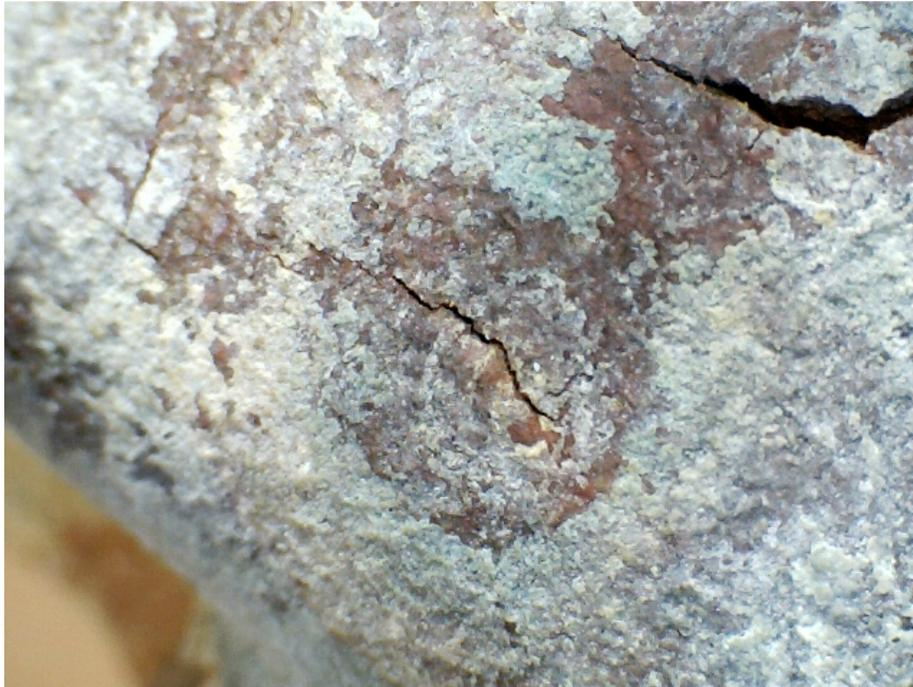
Photo #8 – Dezincification. The white material is zinc oxide that has leached from the alloy. The material has lost substantial strength.
