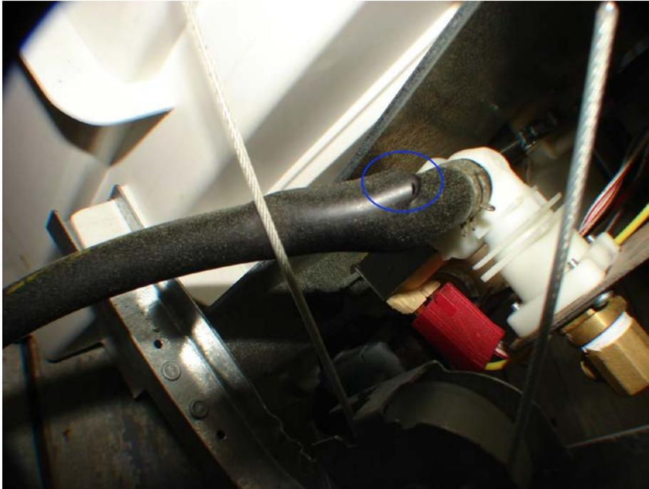
Photo #23 – This water outlet hose from an inlet valve got caught up in the door hinge assembly. The inlet valve had been changed and was installed to put the hose in an improper orientation.
