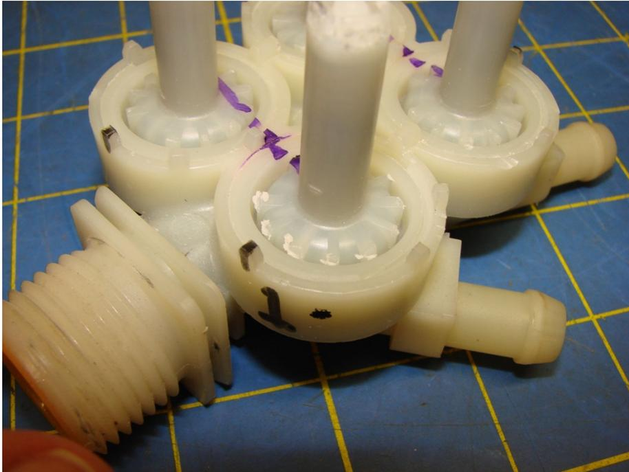
Photo # 13 -- The solenoid has been removed, exposing the valve body. The upper body screws off.
