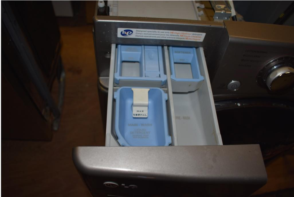
Photo #55 – The detergent dispenser drawer. The inlet valves run cold water through these compartments and into the tub at different times in the cycle.
