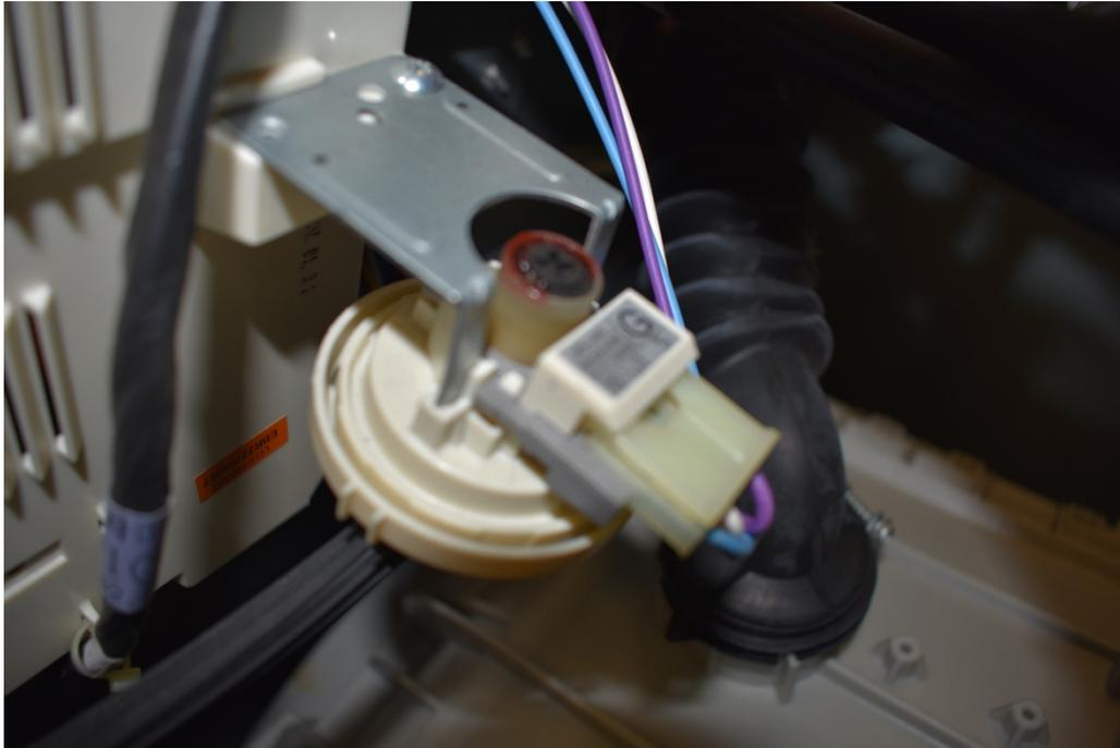
Photo #51 – The pressure sensor shuts off the inlet valve when the water reaches a set level. This is located under the support brace if the photo above.
