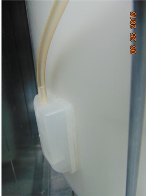
Photo # 44 – At the other end of the system is the air dome and tube connection to the tub. As the water level in the tub increases, the air pressure in the tube increases.
