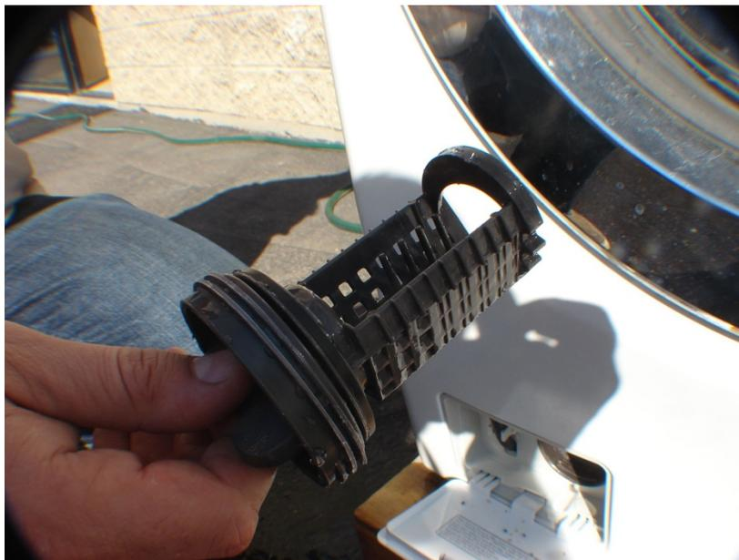
Photo #46 -- This is the filter. It will catch any small clothing items that escape the drum or whatever was left in the pocket of those jeans before the wash. I had one case where a guitar pick blocked the drain just inside the filter cavity.
