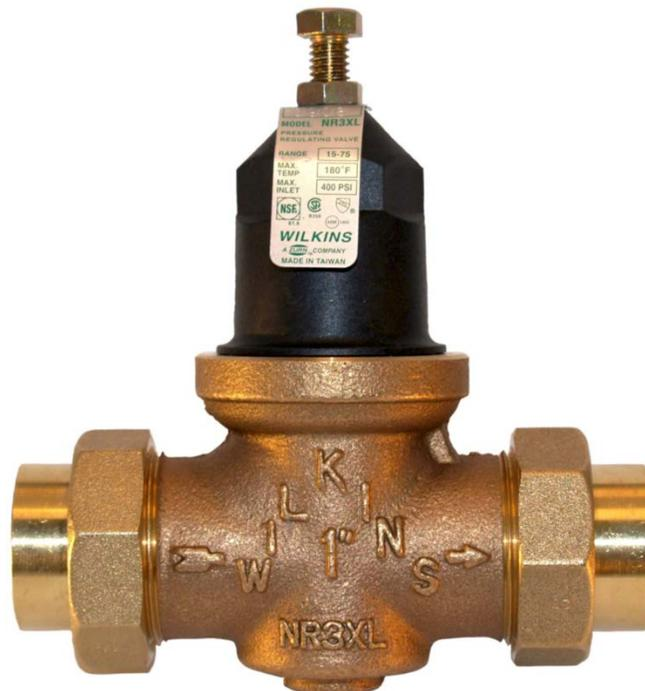
Photo # 1 -- A typical domestic pressure reducing valve. Generally, it can be identified by its shape and will be located just after the whole house shutoff valve. Not all homes have them, and they do require regular testing as they are subject to wear. This valve protects the domestic water system from overpressure.
