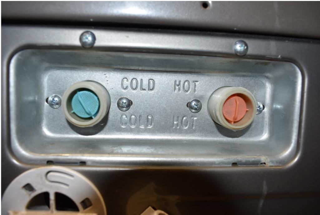
Photo #49 – The hot and cold inlet screens should be checked for debris. Debris may get through and affect the operation of the inlet valve, which has small internal passages.
