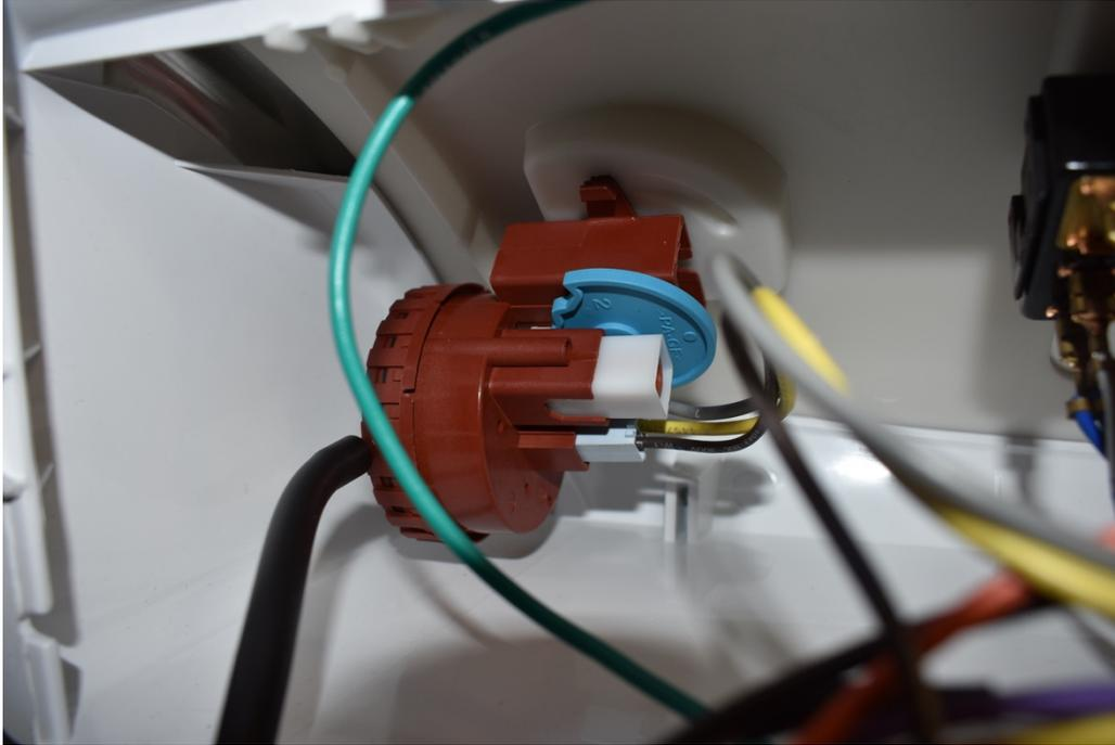
Photo #62 – This is the pressure sensor and water level sensor.
