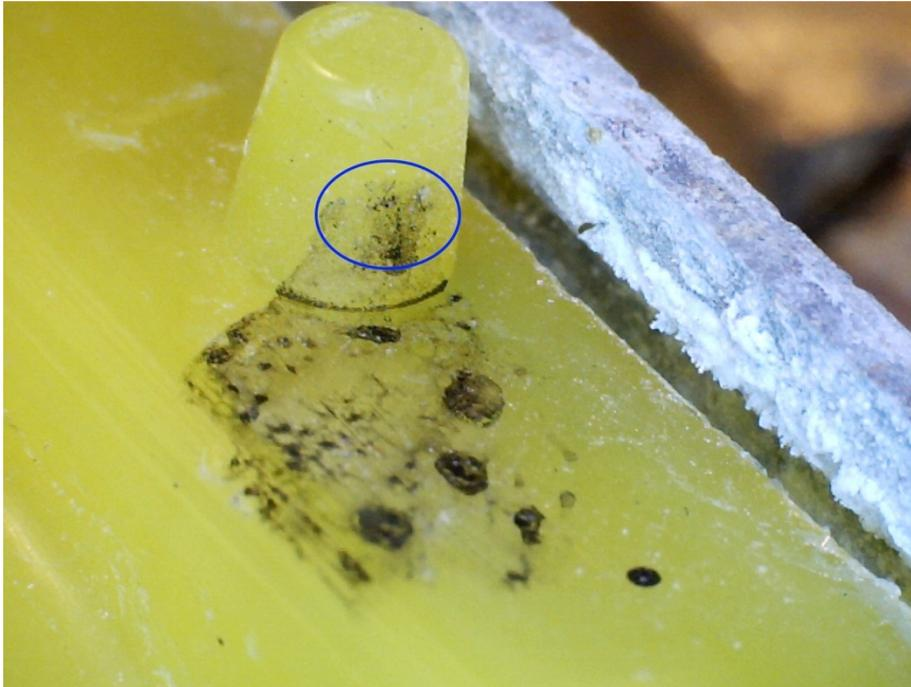
Photo #29 – This one leaked through a defect on the body.
