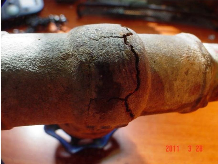
Photo #7 – This is a long-term failure and alloys with greater than 15% zinc content are very susceptible to this form of corrosion. It occurs often when the water has high oxygen and carbon dioxide content.
