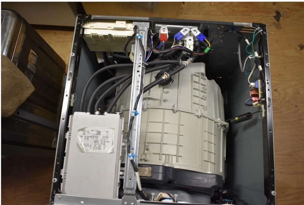
Photo #50 – Removing the top of a front load machine exposes the drum (tub), the electronics (circuit board) package, the detergent dispenser and the noise filter (on the right).
