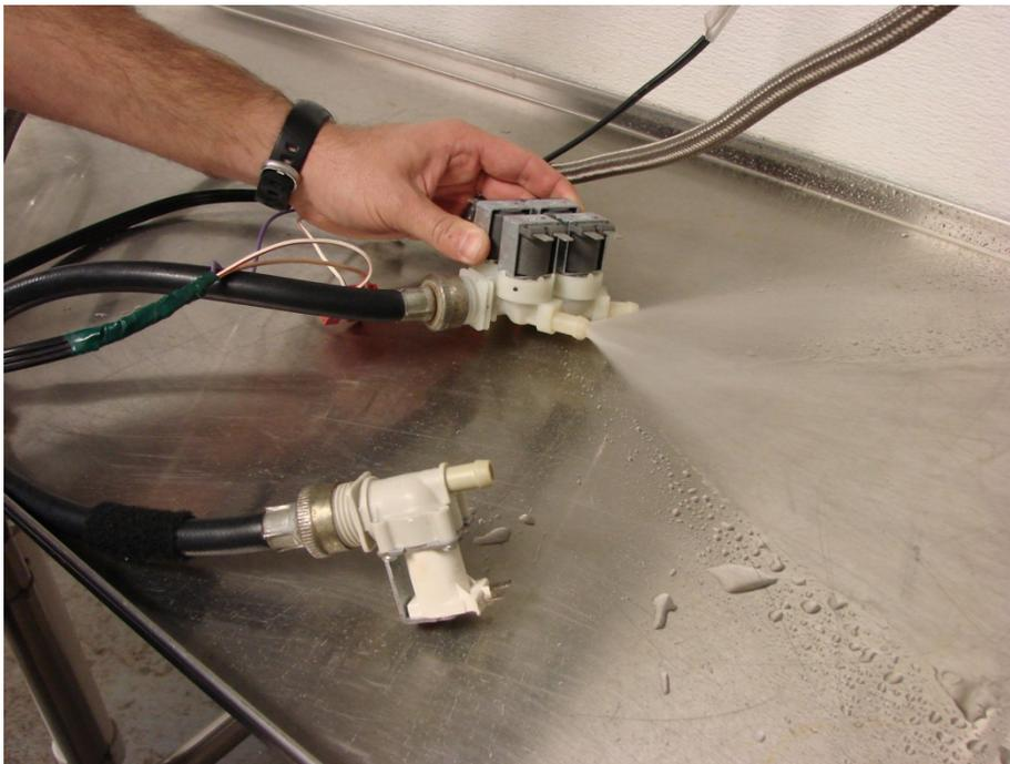
Photo #12 – A ganged solenoid inlet valve set being tested.
