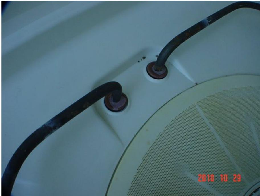
Photo #19 – The heater element in a dishwasher penetrates through the bottom of the tub. These connections show discoloration, but underneath...
