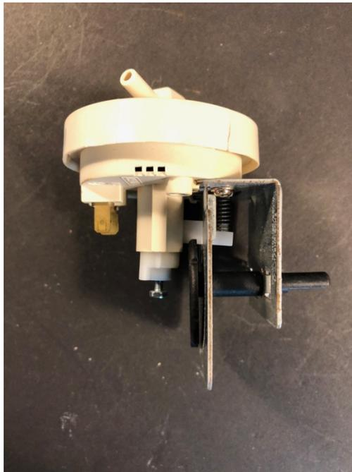
Photo # 39 – A typical pressure sensor/water level valve for a washing machine.
