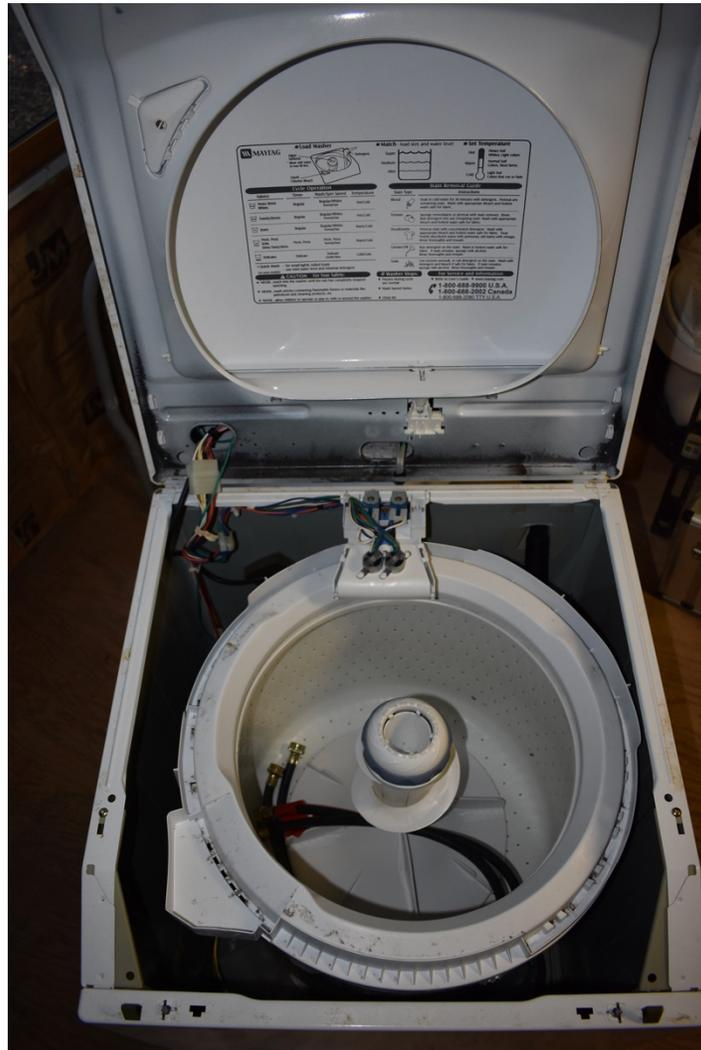
Photo #57 – Opening the top of the machine exposes the tub and agitator. The inlet valves are at the top of the photo.
