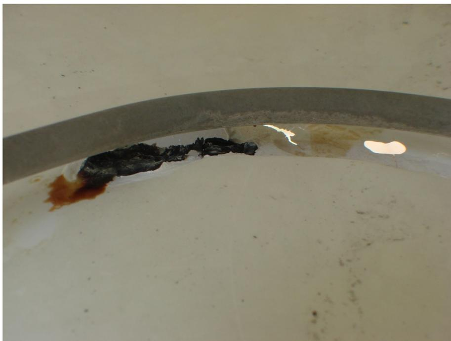
Photo #36 – Contact of a heater element with the plastic tub created a hole in the tub.
