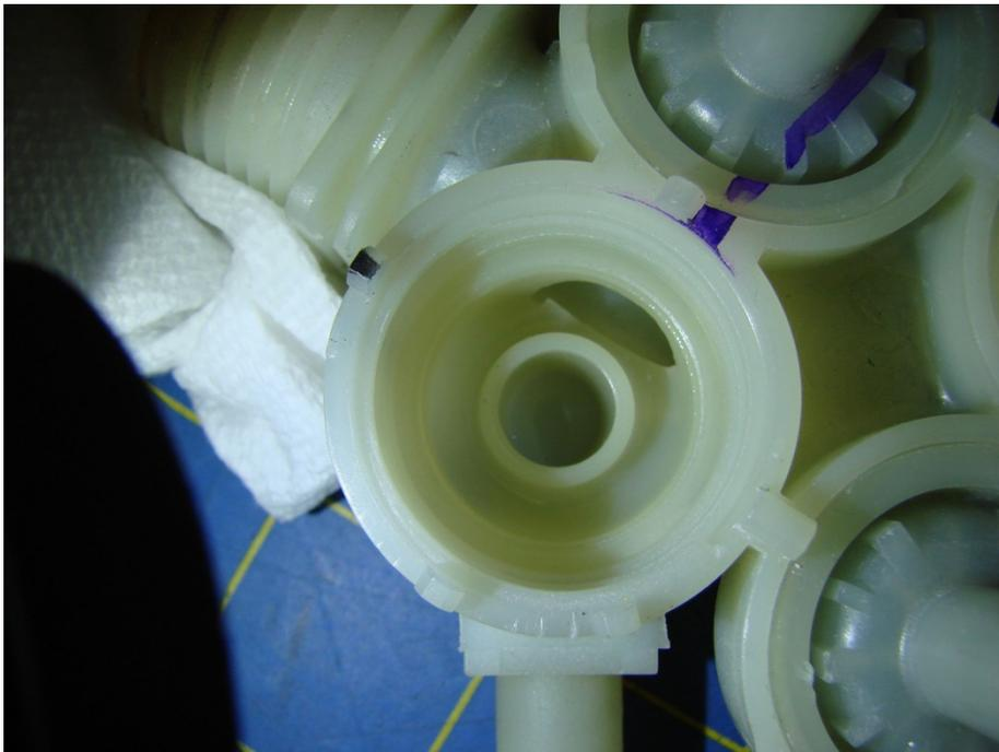
Photo #14 -- The upper body, including the plunger, spring and diaphragm assembly has been removed, showing the lower pressure retaining body and seat of the valve.
