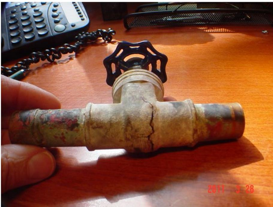
Photo #6 - This is a valve with cracking that results from dezincification.
