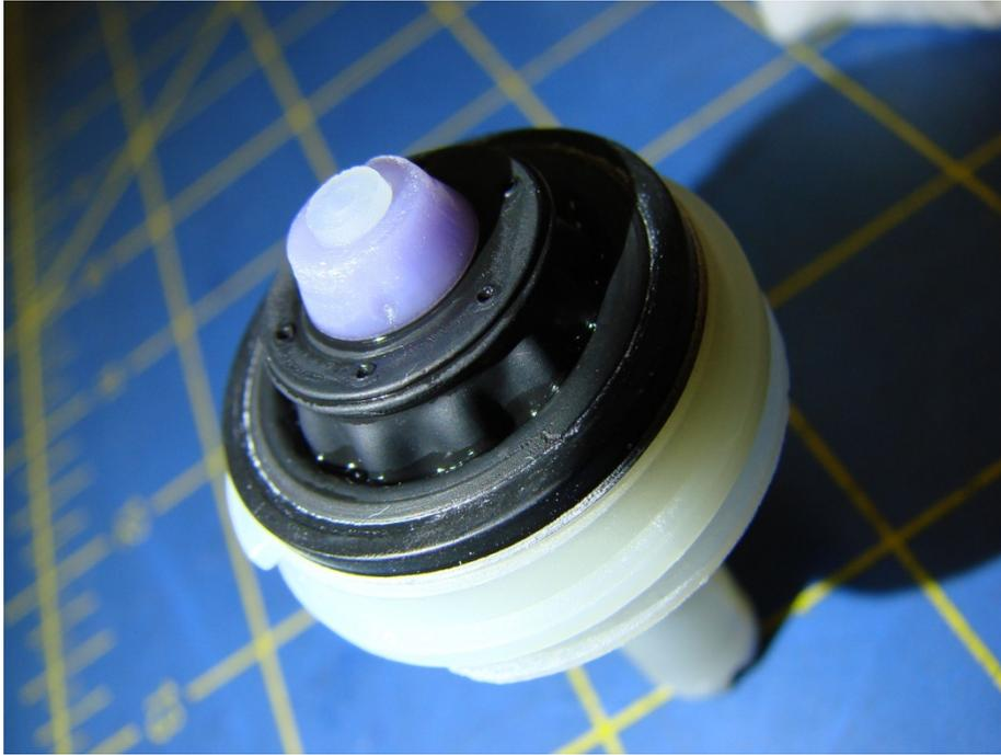
Photo #15 -- The diaphragm assembly. Note the bleed orifices surrounding the purple tip.
