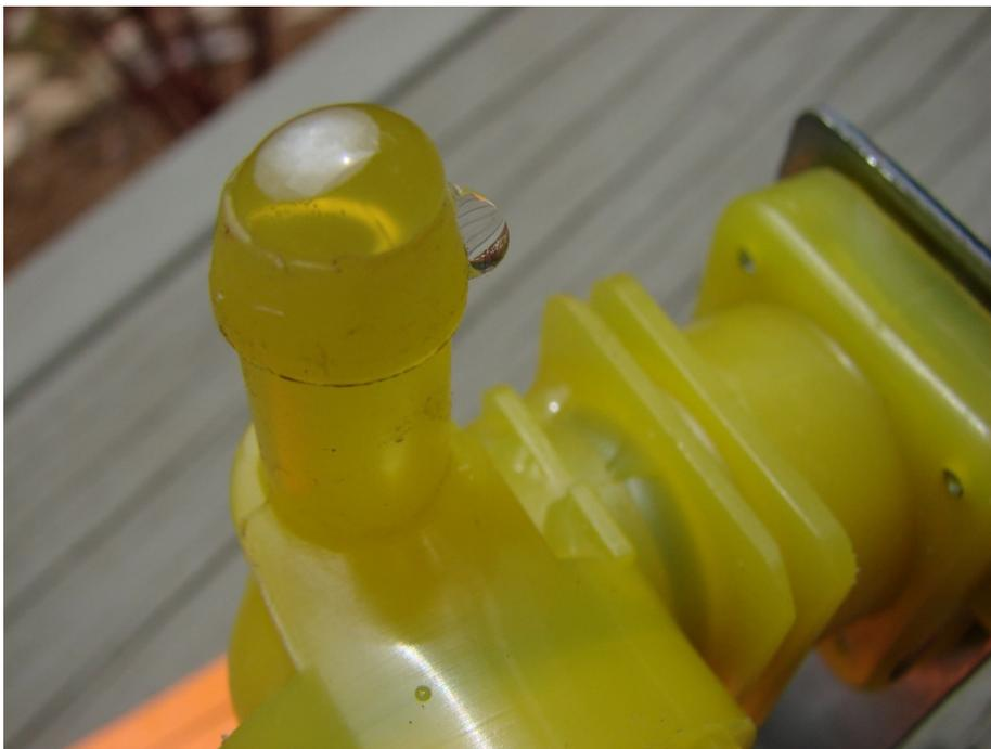
Photo #28 – This inlet valve leaked under water pressure with no power applied.
