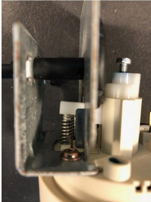
Photo # 40—This mechanism adjusts the set point as one rotates the selection valve to different cycles that are associated with different water heights. The black shaft is rotated by the used to select the cycle. The shaft wheel is configured to set the contact distance.
