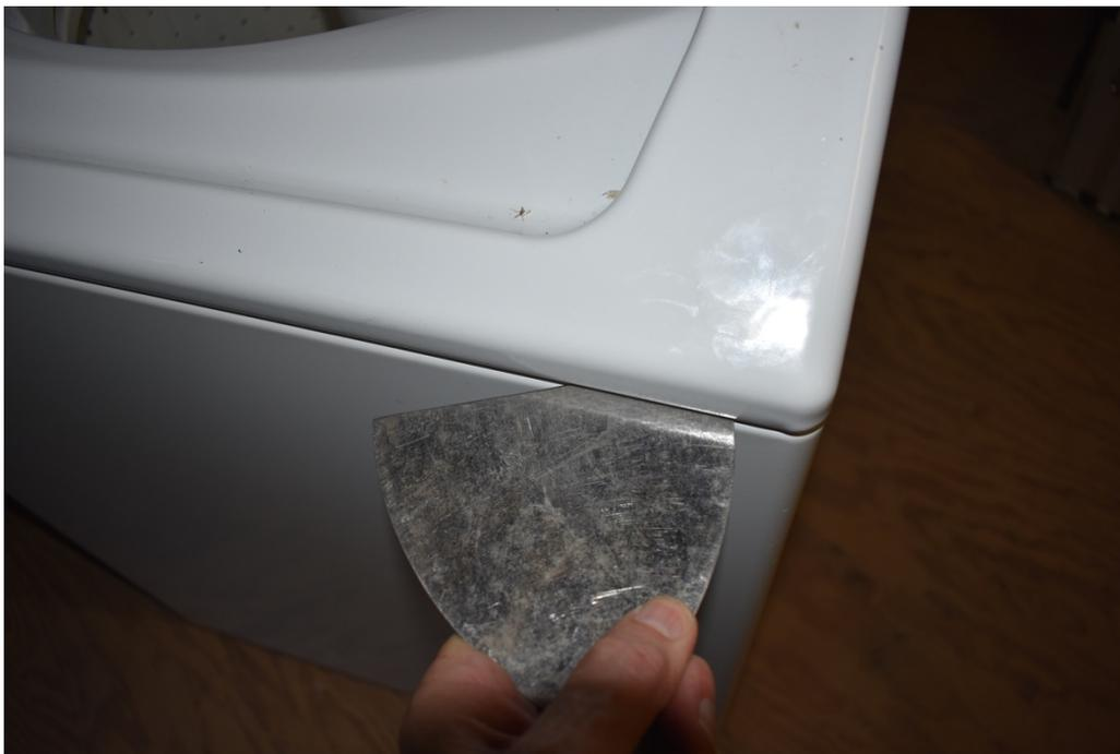
Photo #56 – On a top load machine, the top or side latches are often hidden. Pushing a putty knife in a little does the job.
