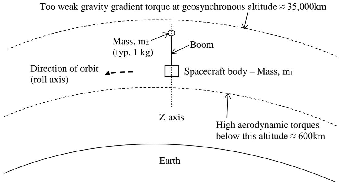
**Figure 2.5: Gravity Gradient Stabilization**
