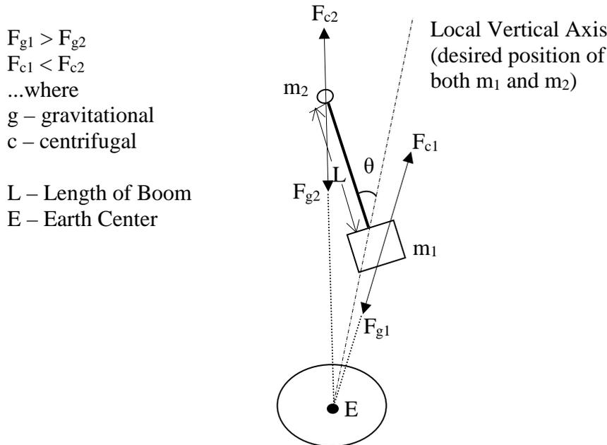
**Figure 2.6: Gravity Gradient Forces**
