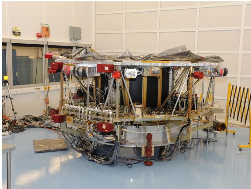
**Figure 2.3: MMS Spacecraft Structure – AFTER Subsystem Integration**
