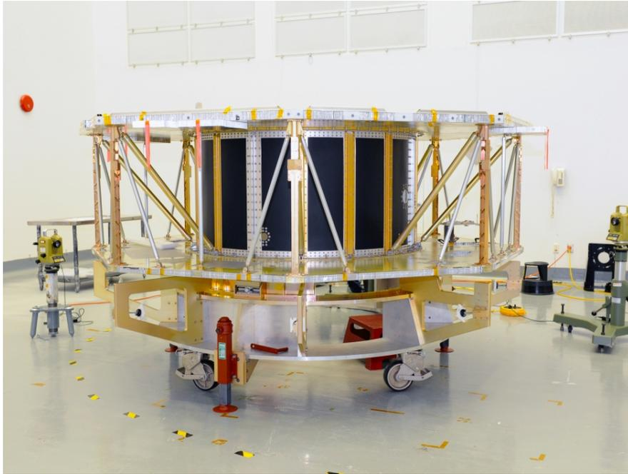
**Figure 2.2: MMS Spacecraft Structure – BEFORE Subsystem Integration**
