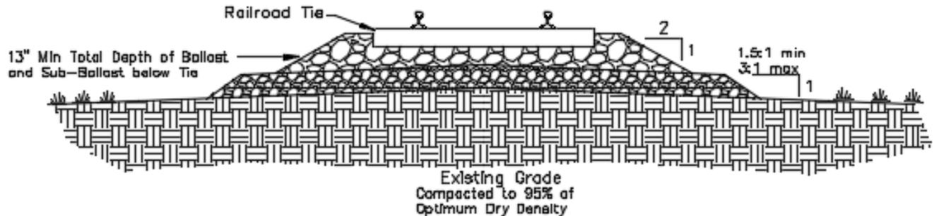
Figure 11 - Example for Light Rail Transit Track Cross-section
