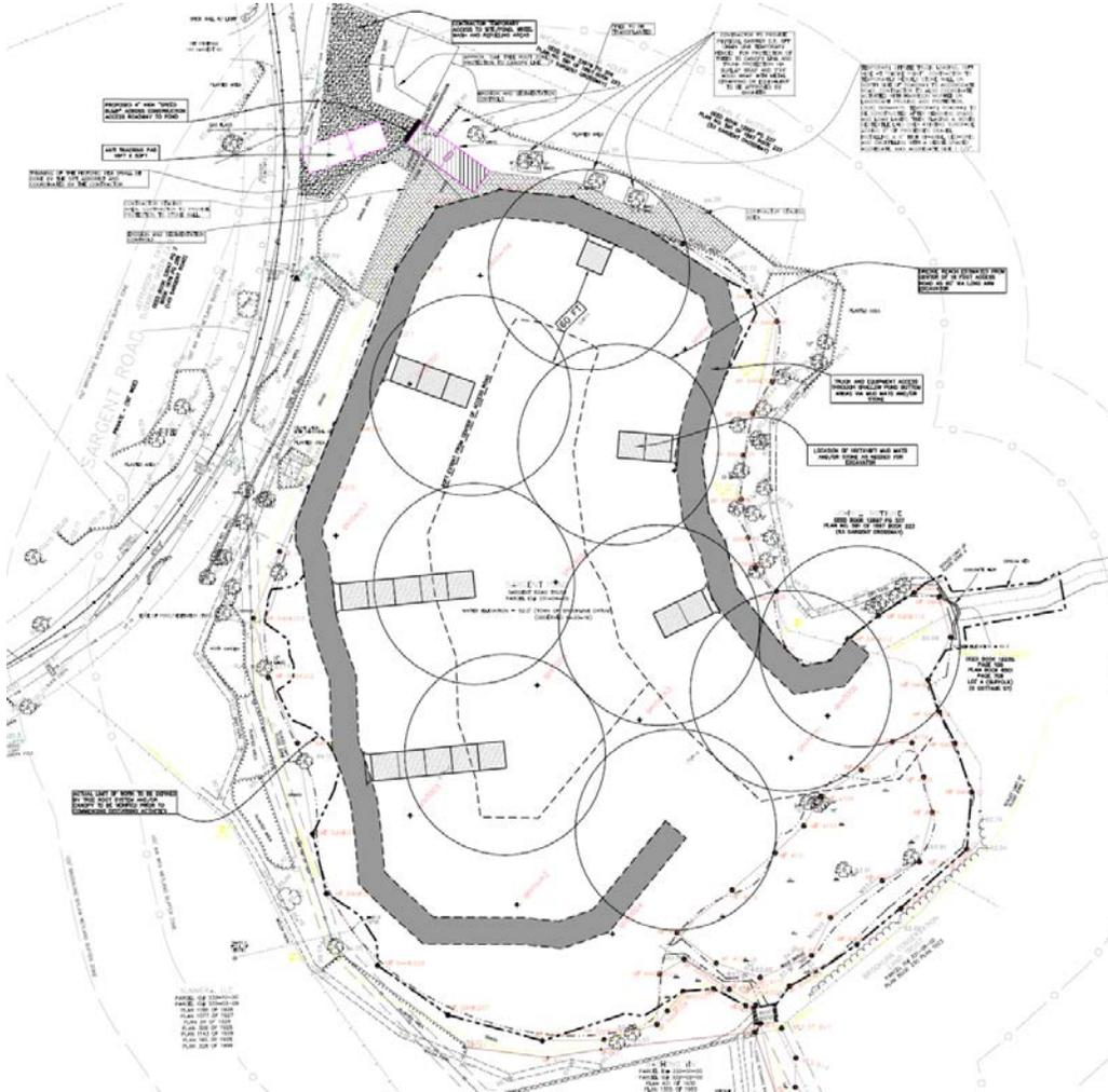
This figure shows the perimeter roadway that traverse the pond and the fingers that provide access for the excavators to dredge. The circles represent the radius of reach for excavators. This figure shows that with some planning, the contractor will be able to dredge the entire footprint without having to crisscross the pond or lay mud mats everywhere.
